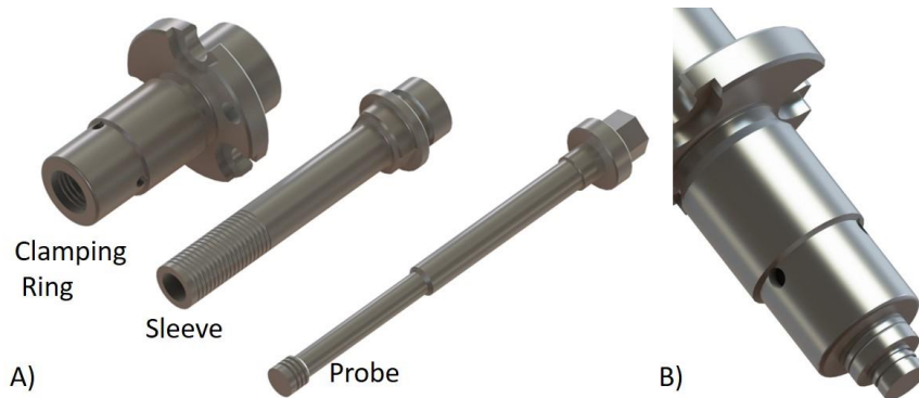
Figure 2.1. A) Schematic of the refill FSSW tool. B) Assembly of the refill FSSW tool.
