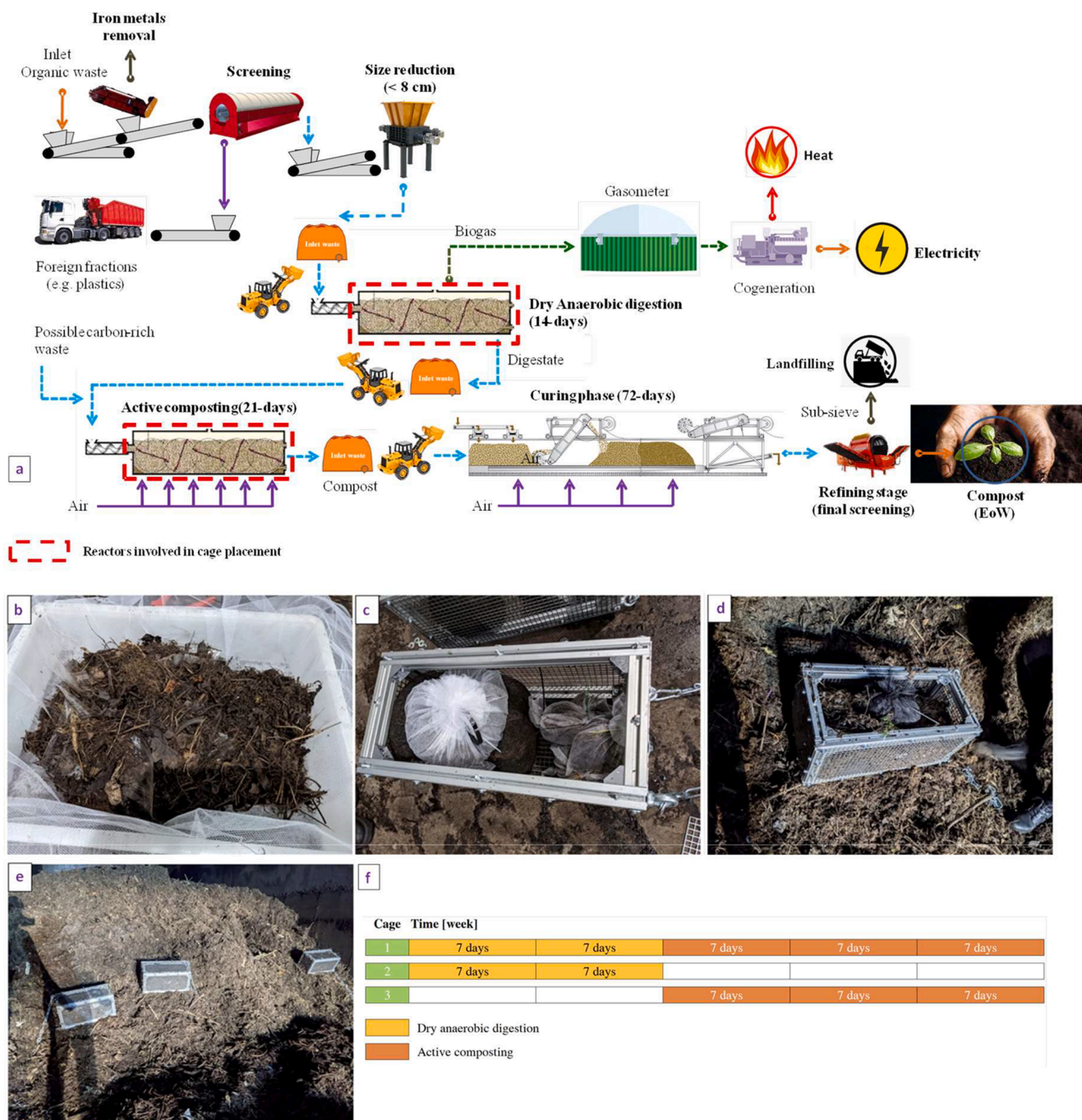
Fig. 1. Full-scale plant layout with reactors involved in cage placement (a); Cages preparation and positioning: (b) mixture of CA based samples with separate collected biowaste/digestate, (c) placing the net in the metal cage, (d-e) placing the cages in the biomass to process and covering them; Experimentation timeline (f). Single images with higher resolution are shown in Supplementary Materials.
