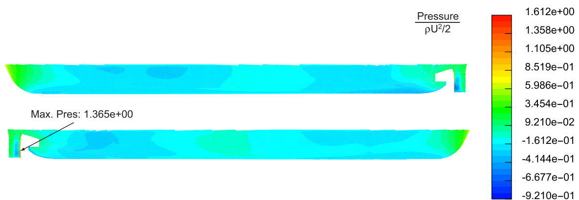
Figure 6.26: Dynamic pressure distribution on the ship hull and the rudder surface of the CBOX ship at \psi = 10^\circ during the Zigzag maneuver, viewed from port side (top) and starboard (bottom).
