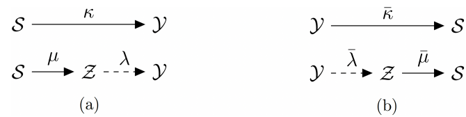
Figure 2. (a) Simulation of the channel \kappa through a randomization at the output of \mu , where \kappa and \mu share a common input alphabet \mathcal{S} . (b) Simulation of the channel \bar{\kappa} through a randomization at the input of \bar{\mu} , where \bar{\kappa} and \bar{\mu} share a common output alphabet \mathcal{S} .
