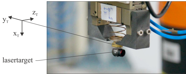
Fig. 6. Lasertarget attached to an insert
