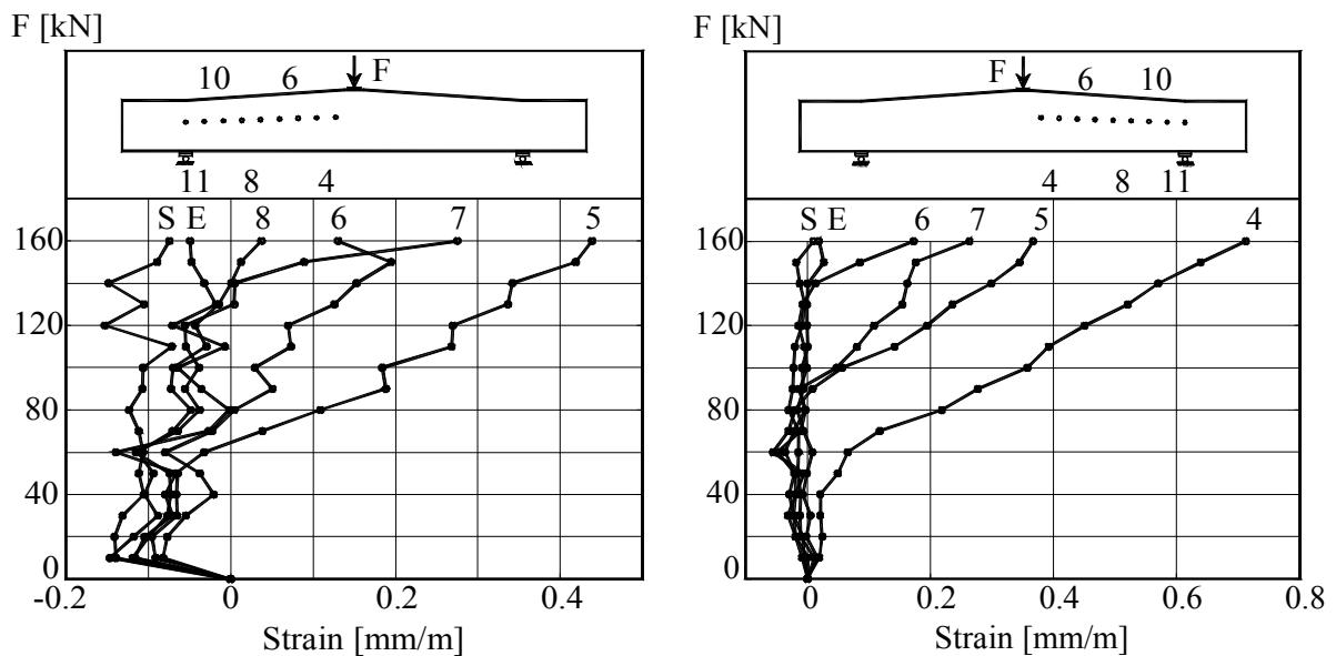
Figure B.2K1.6- The Load –Strains graph at mid-depth of beam
