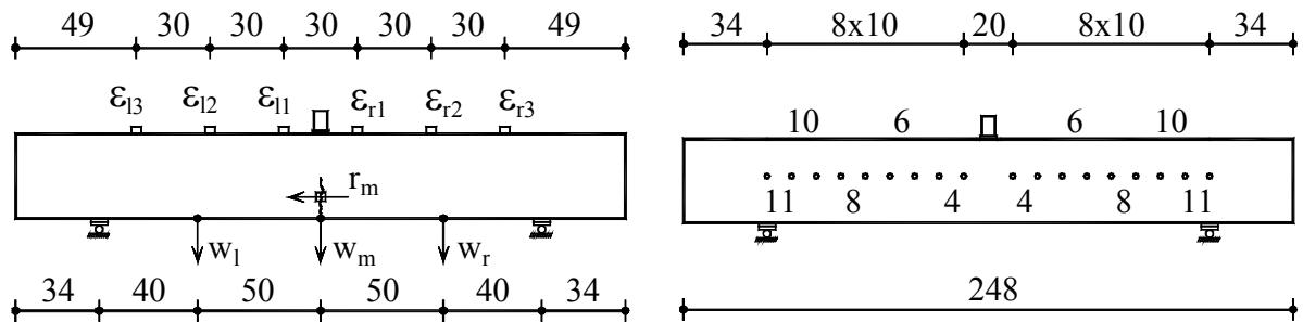
Figure B.1K2.1- The detailed arrangement of the data acquisition system
