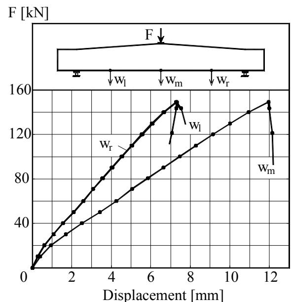
Figure B.2L2.3–The Load – Displacement graph
