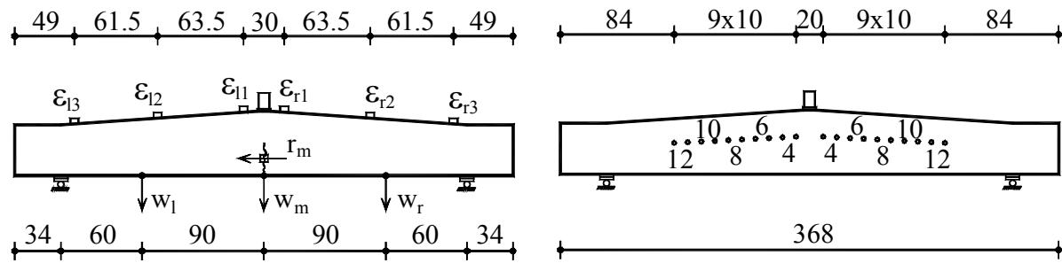
Figure B.2L1.1 – The detailed arrangement of the data acquisition system
