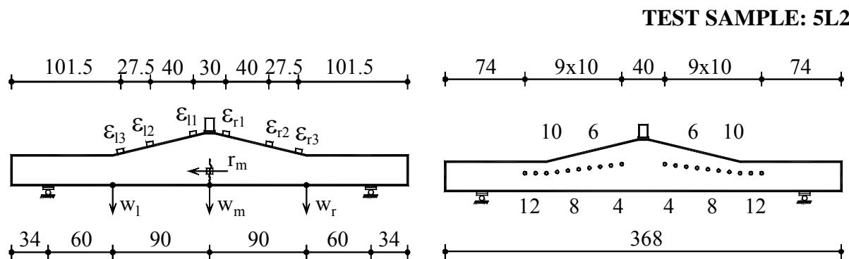
Figure B.5L2.1- The detailed arrangement of the data acquisition system
