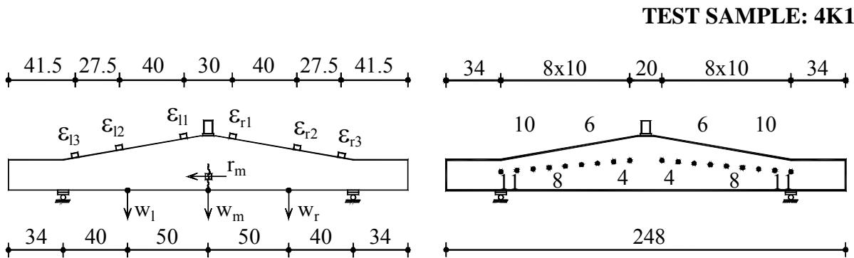
Figure B.4K1.1- The detailed arrangement of the data acquisition system
