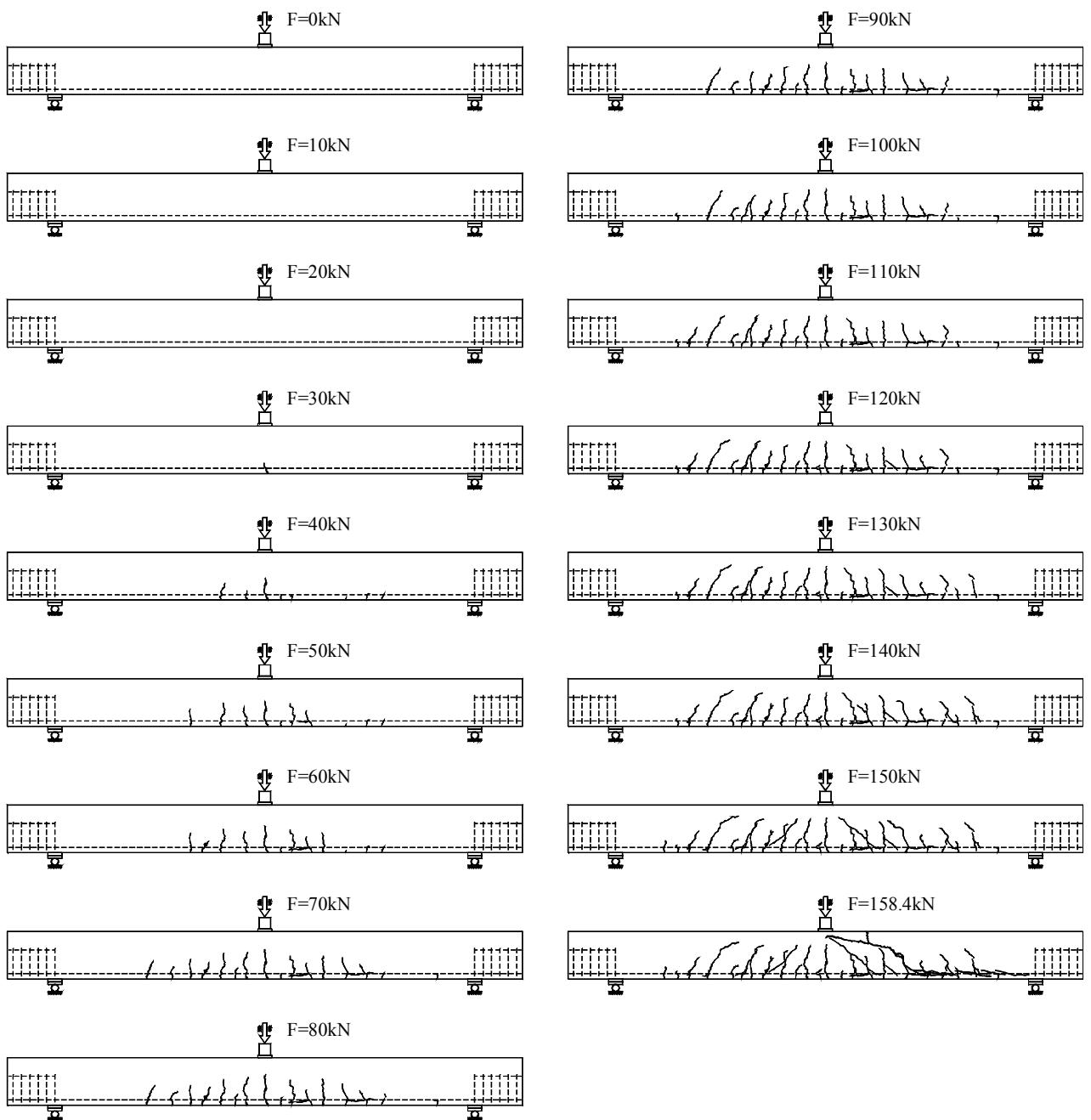
Figure B.1L2.7– Crack propagation of beam 1L2 after each load step.
