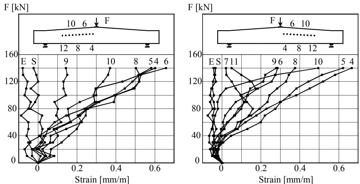
Figure B.2L2.6 – The Load –Strains graph at mid-depth of beam
