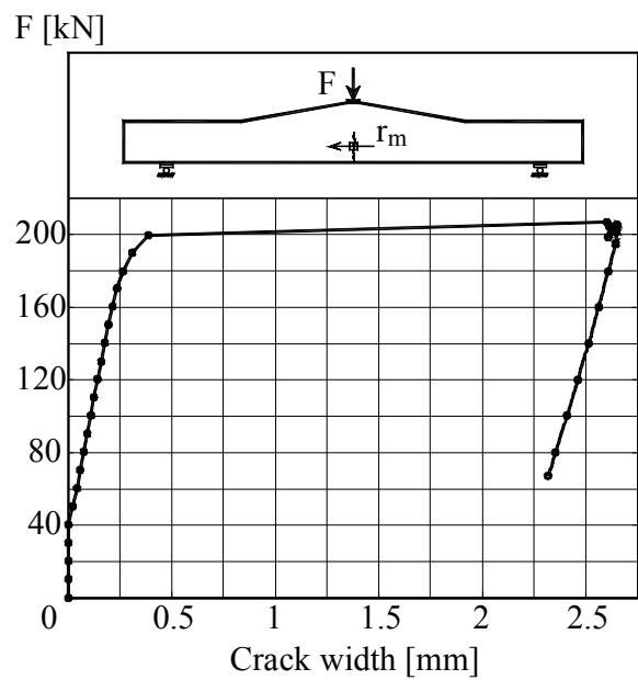
Figure B.4L1.4-The load – crack width graph
