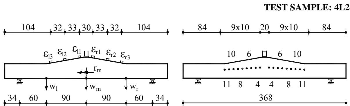
Figure B.4L2.1- The detailed arrangement of the data acquisition system
