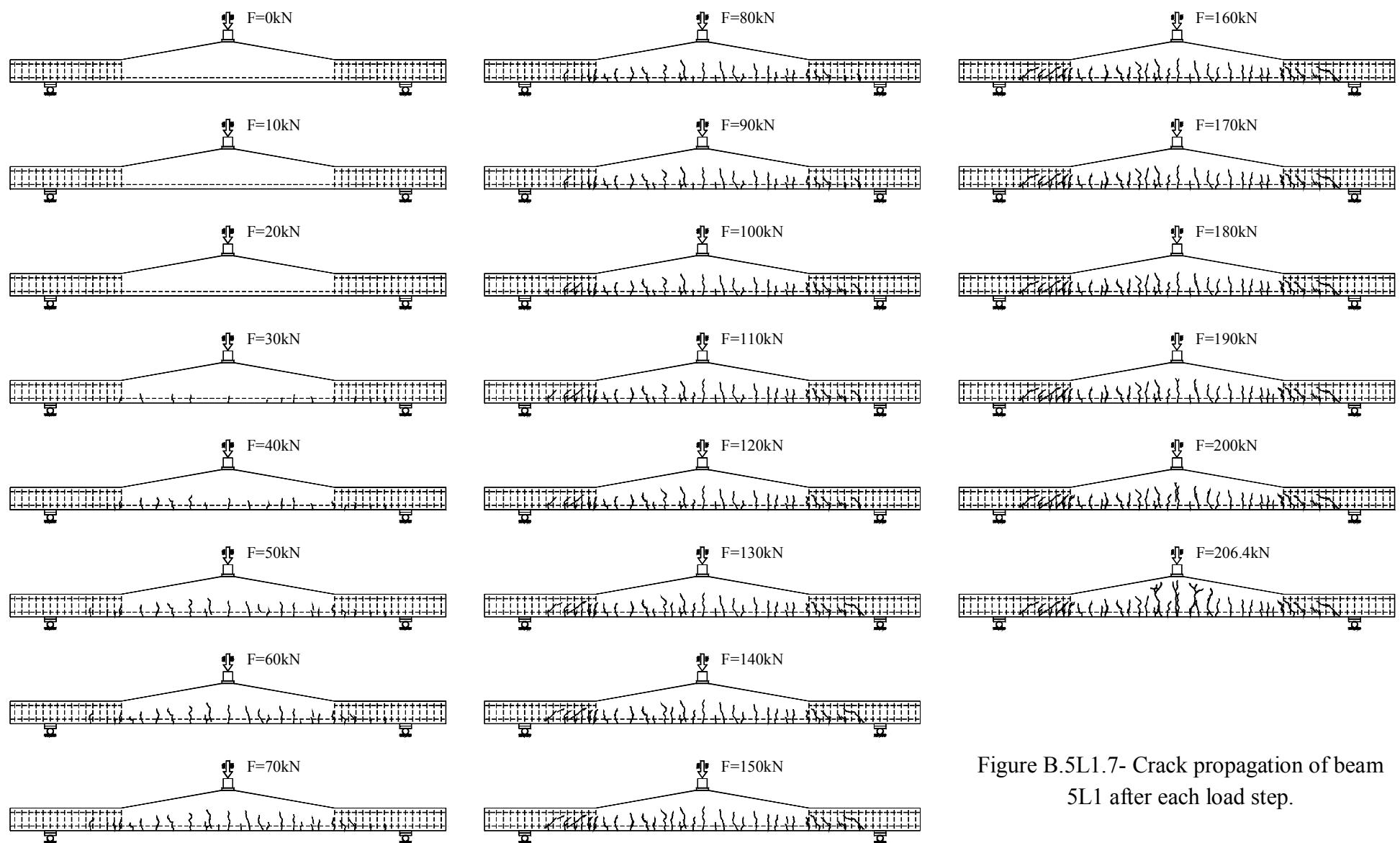
Figure B.5L1.7- Crack propagation of beam 5L1 after each load step.
