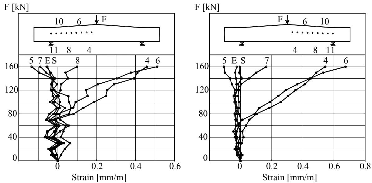
Figure B.2K2.6- The Load –Strains graph at mid-depth of beam
