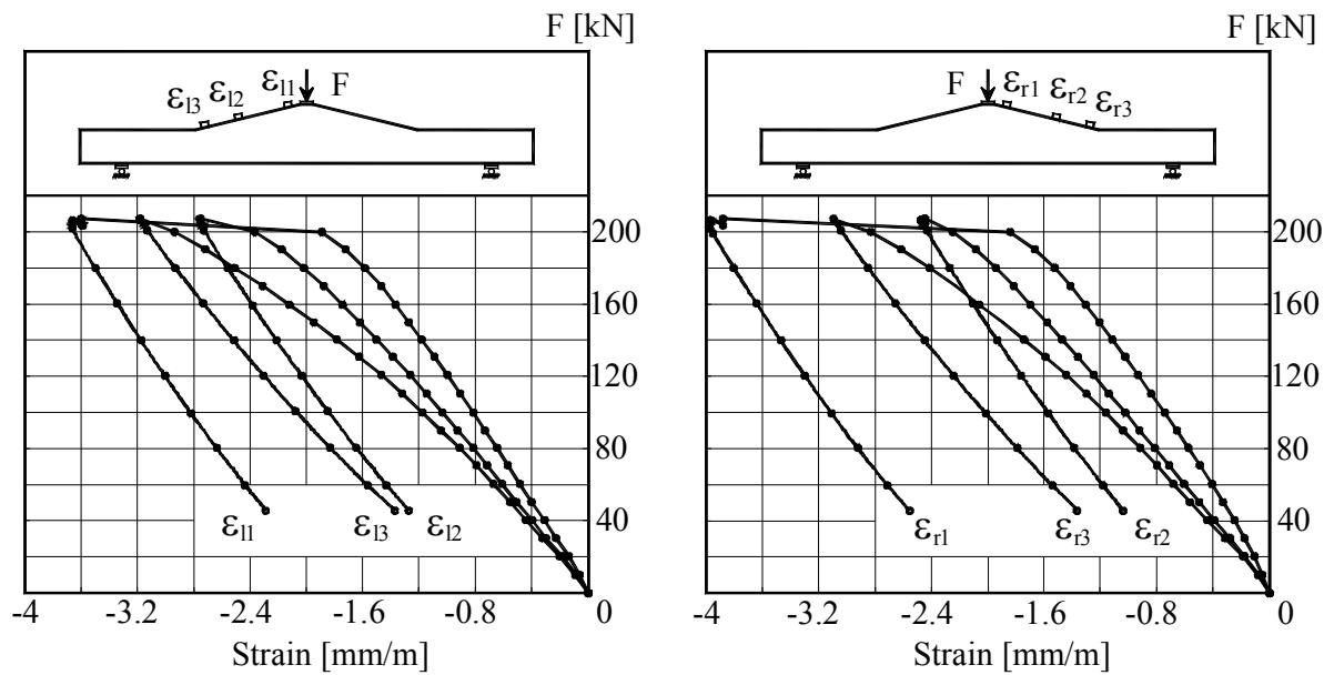
Figure B.5L2.5-The Load –Strains graph at top surface of beam
