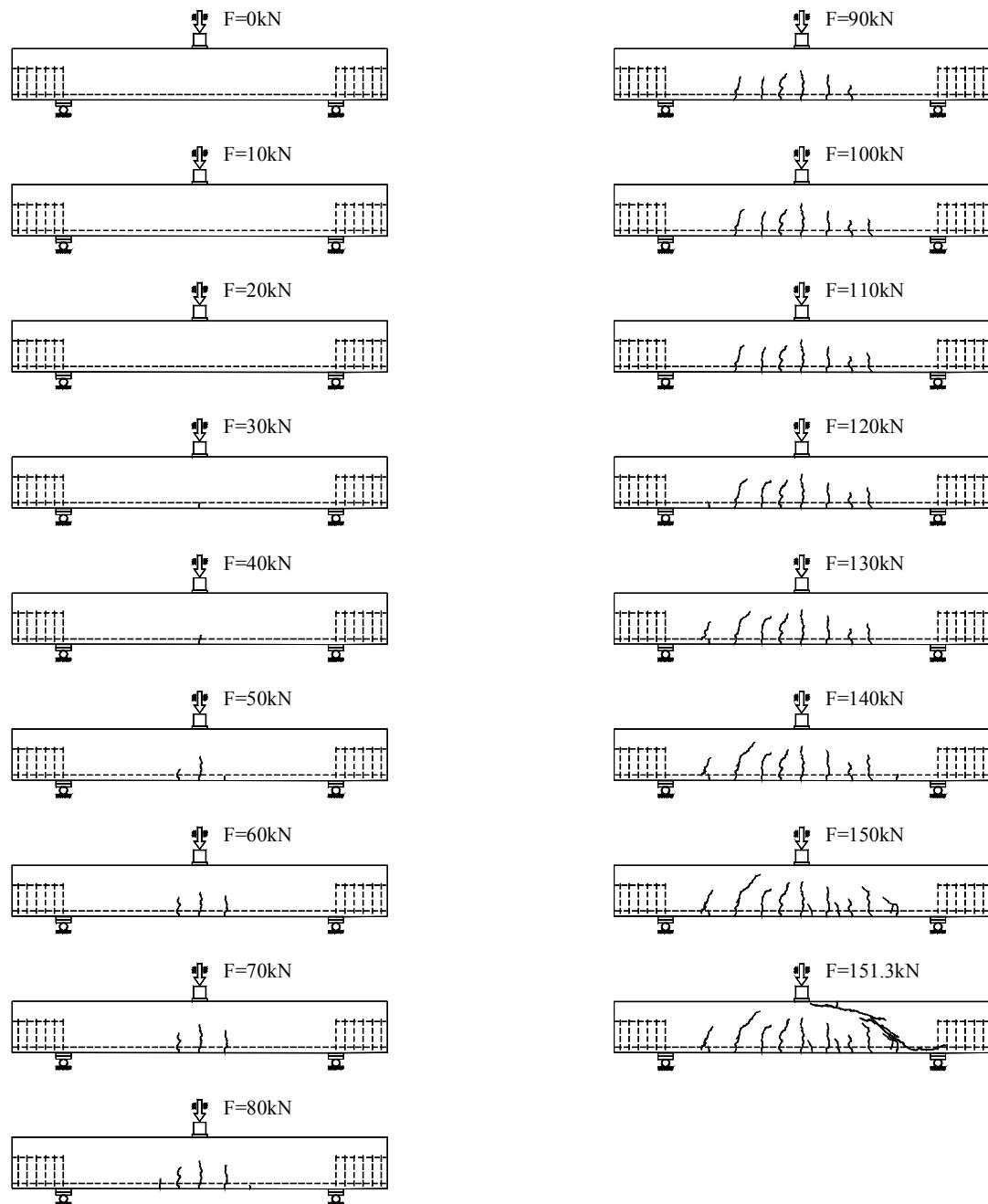
Figure B.1K1.7- Crack propagation of beam 1K1 after each load step.
