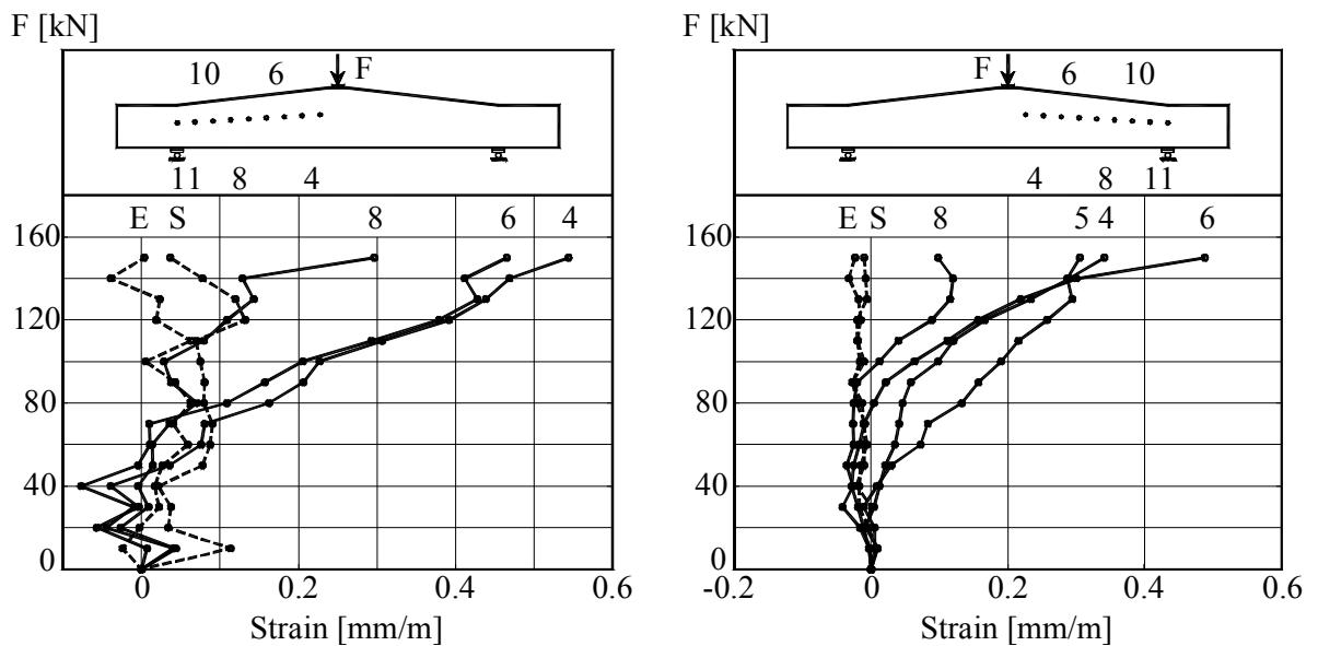
Figure B.3K1.6- The Load –Strains graph at mid-depth of beam
