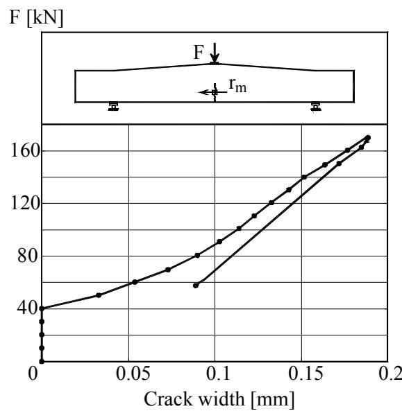
Figure B.2K2.4-The load – crack width graph
