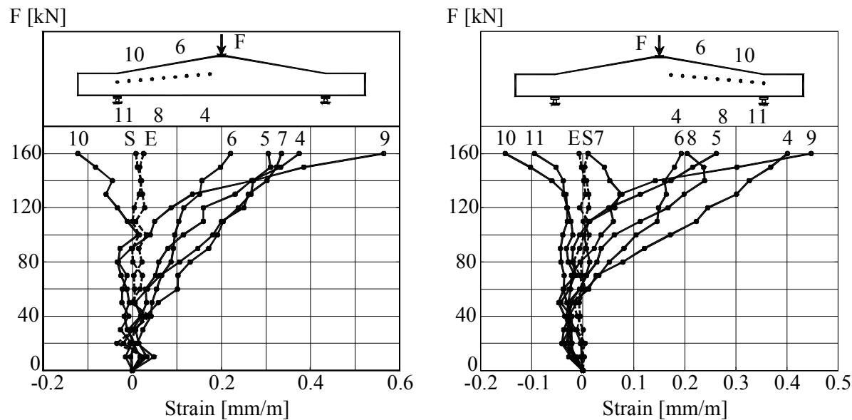
Figure B.4K2.6- The Load –Strains graph at mid-depth of beam
