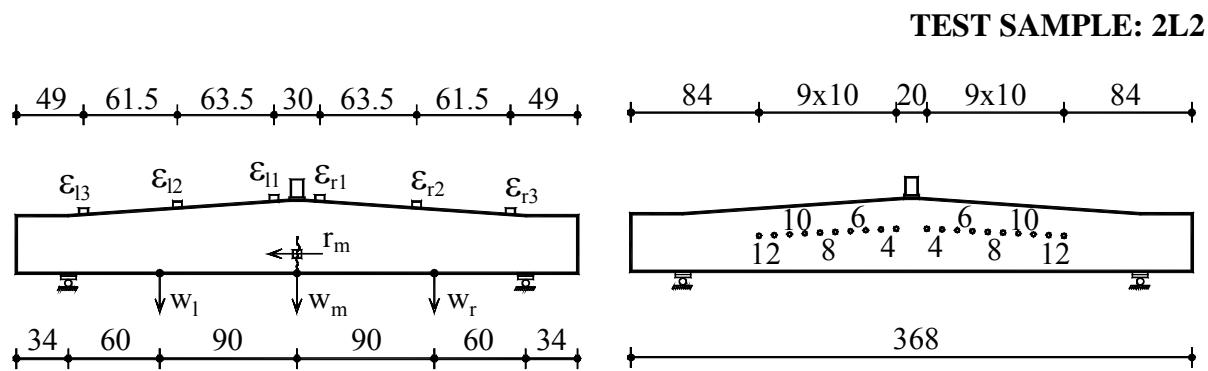
Figure B.2L2.1– The detailed arrangement of the data acquisition system
