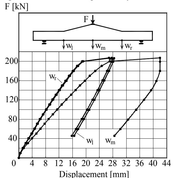
Figure B.5L2.3-The Load – Displacement graph
