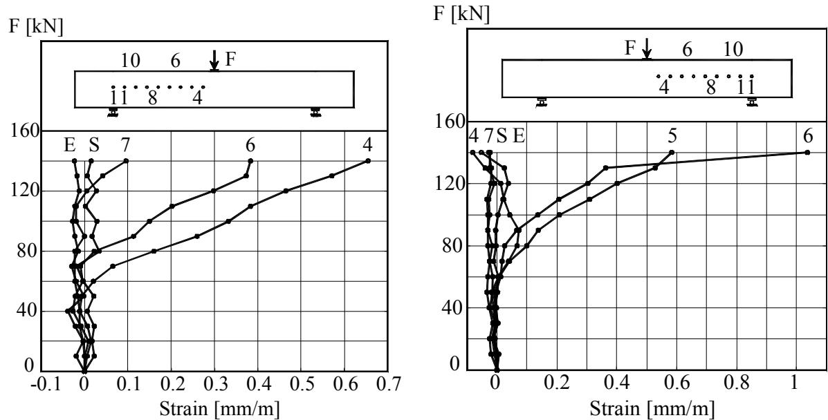
Figure B.1K2.6- The Load –Strains graph at mid-depth of beam
