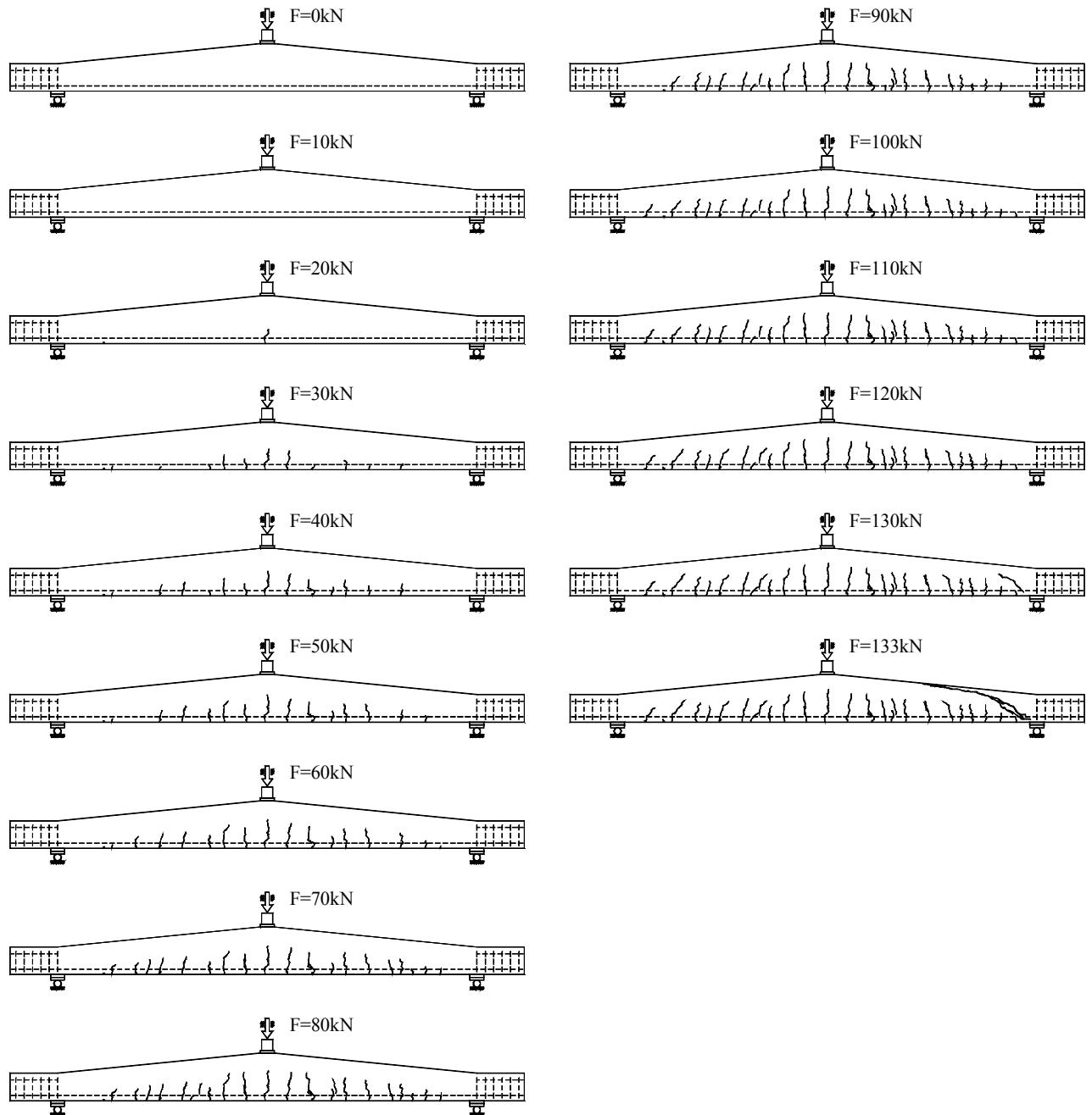
Figure B.3L1.7– Crack propagation of beam 3L1 after each load step.
