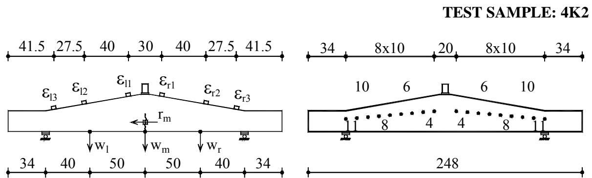
Figure B.4K2.1- The detailed arrangement of the data acquisition system
