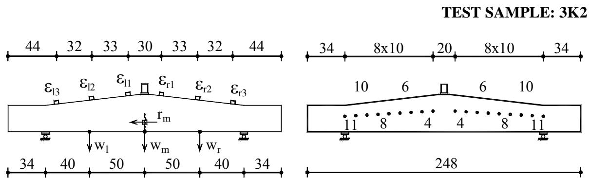
Figure B.3K2.1- The detailed arrangement of the data acquisition system
