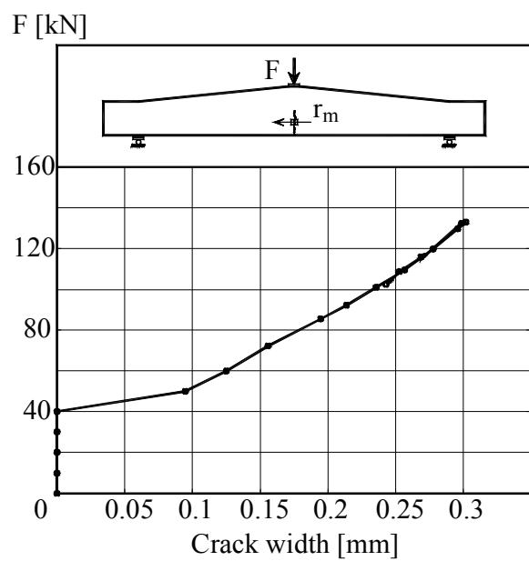
Figure B.3L1.4–The load – crack width graph
