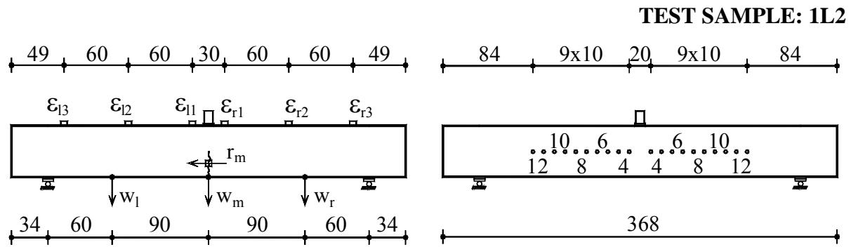
Figure B.1L2.1– The detailed arrangement of the data acquisition system
