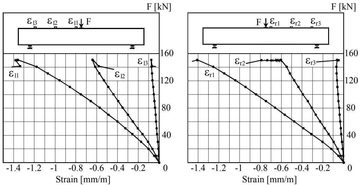
Figure B.1L1.4– The Load – Strains graph at top surface of beam
