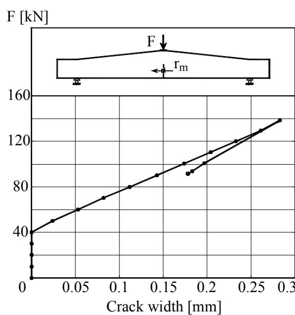
Figure B.3L2.4-The load – crack width graph
