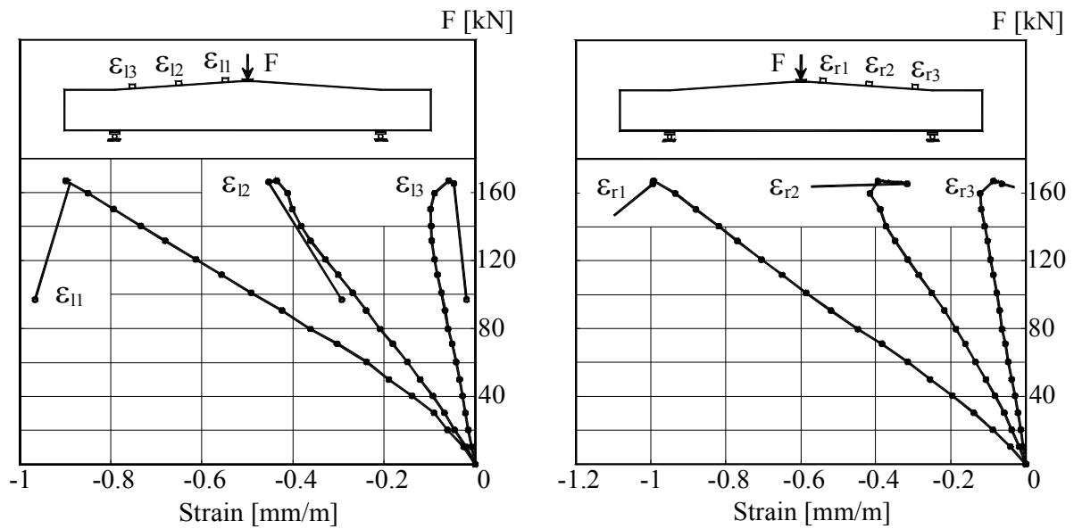
Figure B.2K1.5-The Load –Strains graph at top surface of beam
