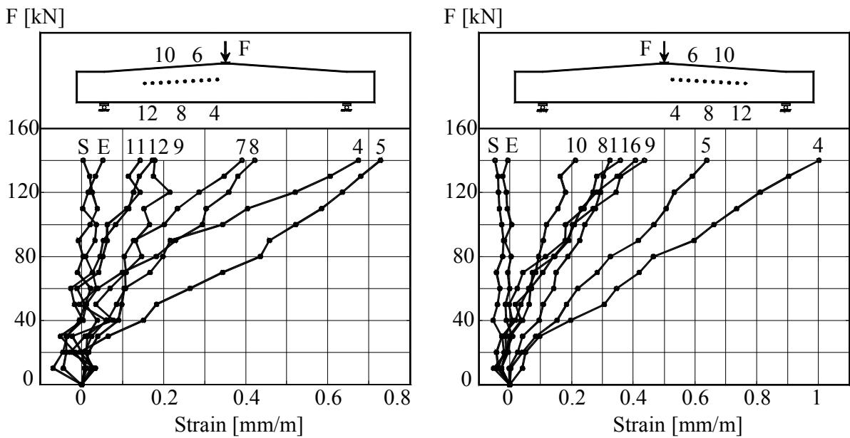
Figure B.2L1.6– The Load –Strains graph at mid-depth of beam
