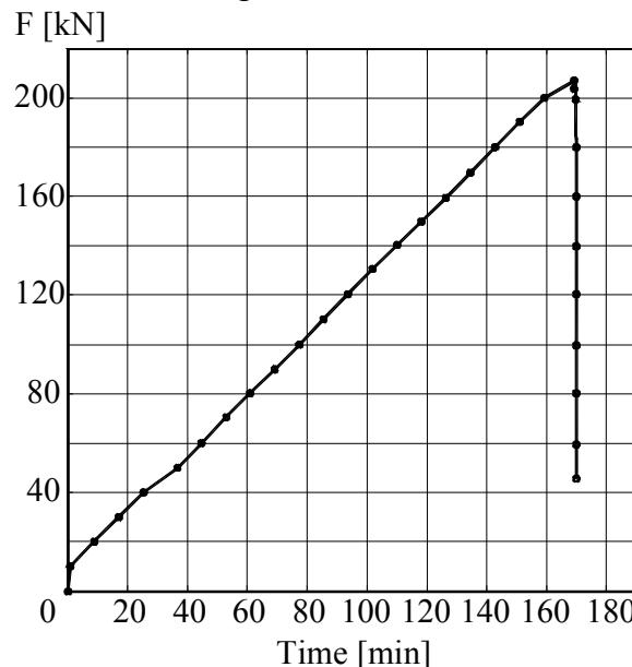
Figure B.5L2.2-The Time – Load graph
