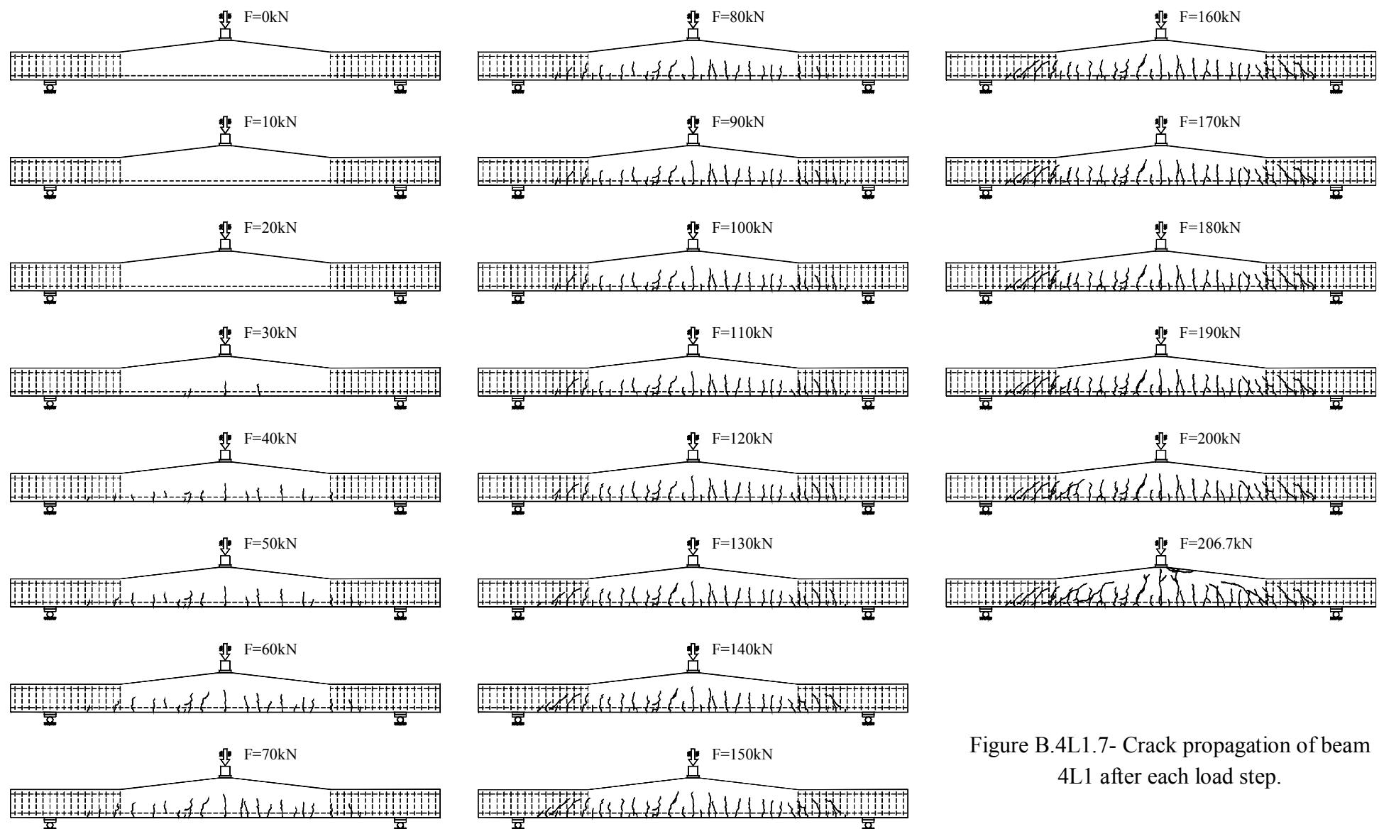
Figure B.4L1.7- Crack propagation of beam 4L1 after each load step.
