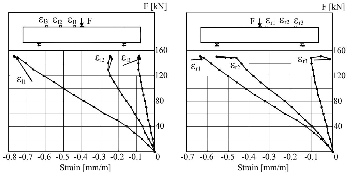
Figure B.1K1.5-The Load –Strains graph at top surface of beam
