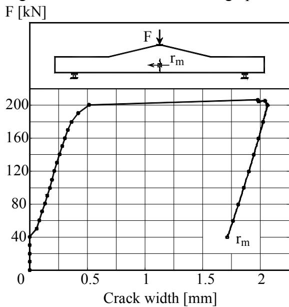
Figure B.5L1.4-The load – crack width graph
