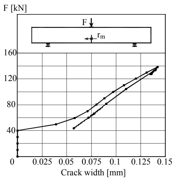
Figure B.1K2.4-The load – crack width graph
