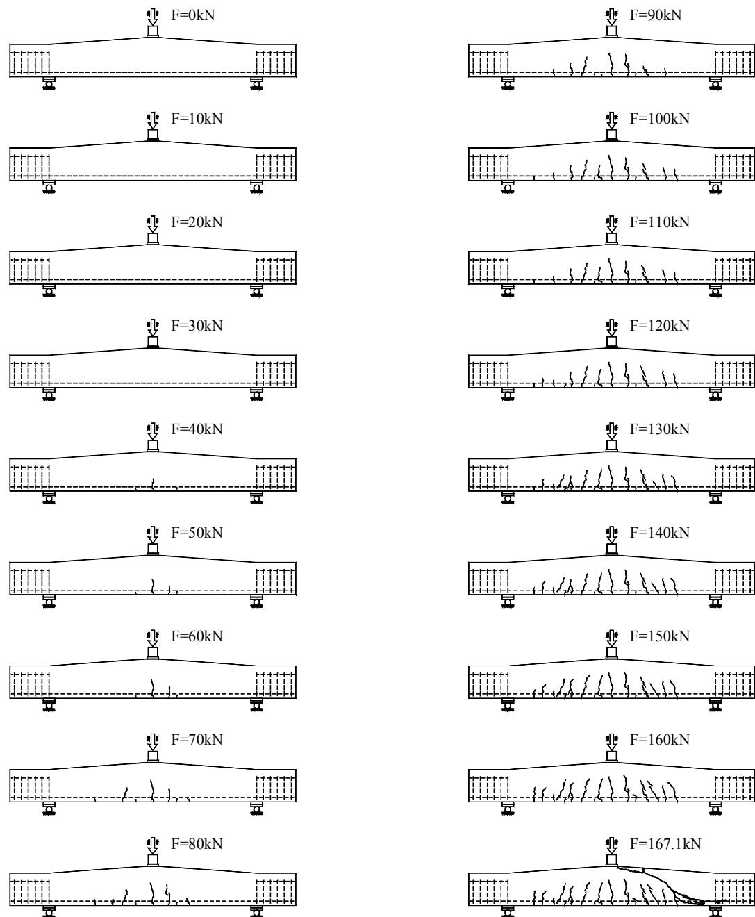
Figure B.2K1.7- Crack propagation of beam 2K1 after each load step.
