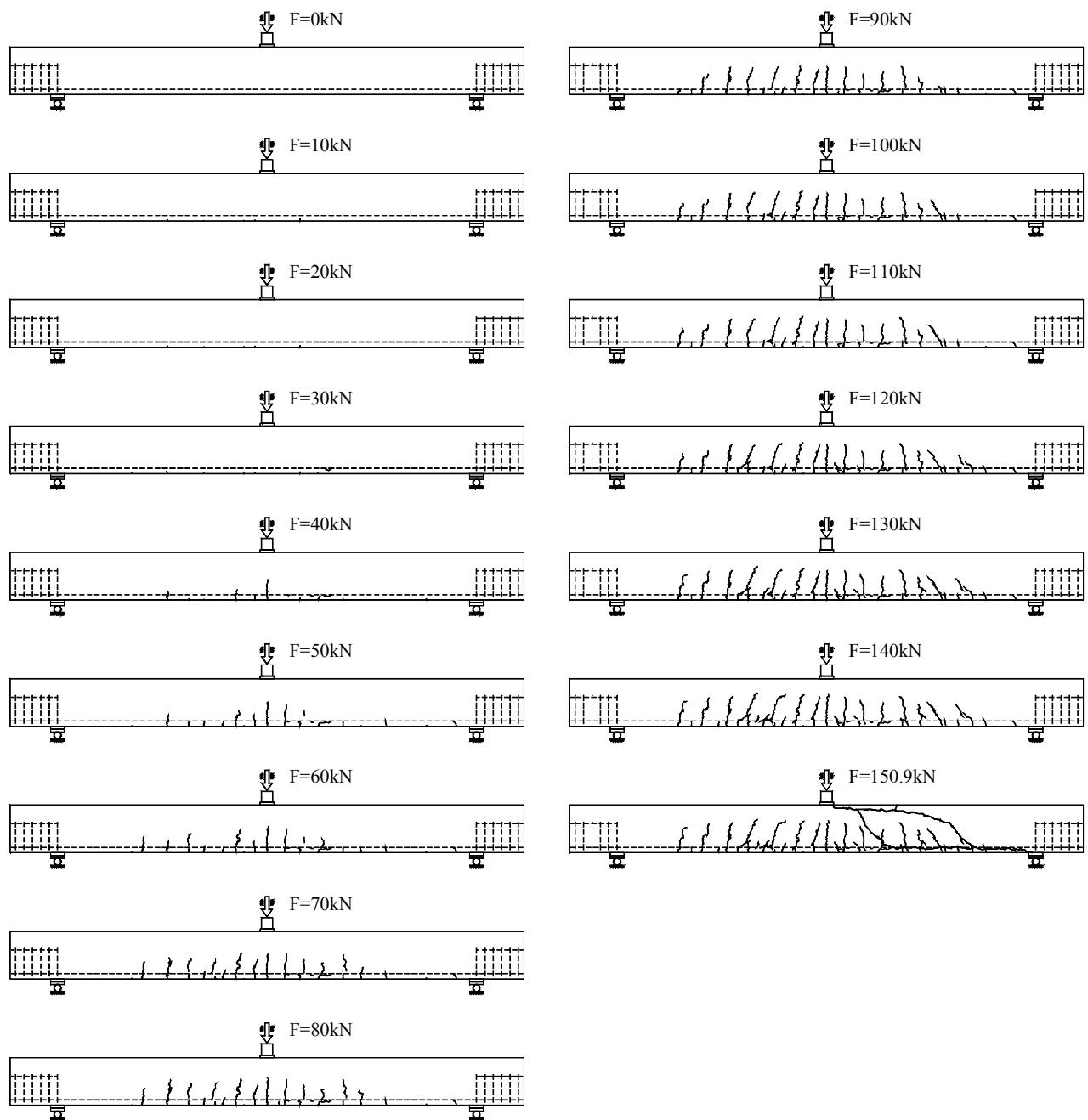
Figure B.1L1.6– Crack propagation of beam 1L1 after each load step.
