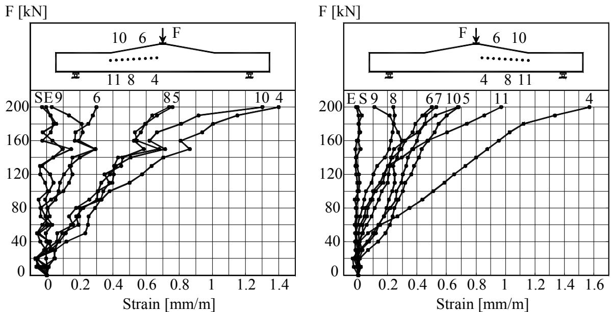
Figure B.4L1.6- The Load –Strains graph at mid-depth of beam
