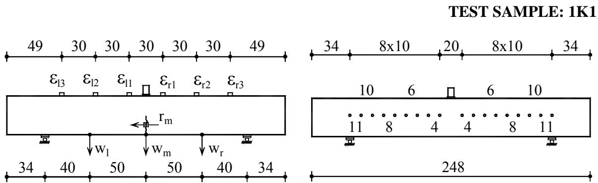
Figure B.1K1.1- The detailed arrangement of the data acquisition system
