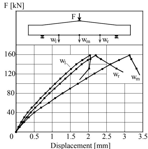
Figure B.3K1.3-The Load – Displacement graph
