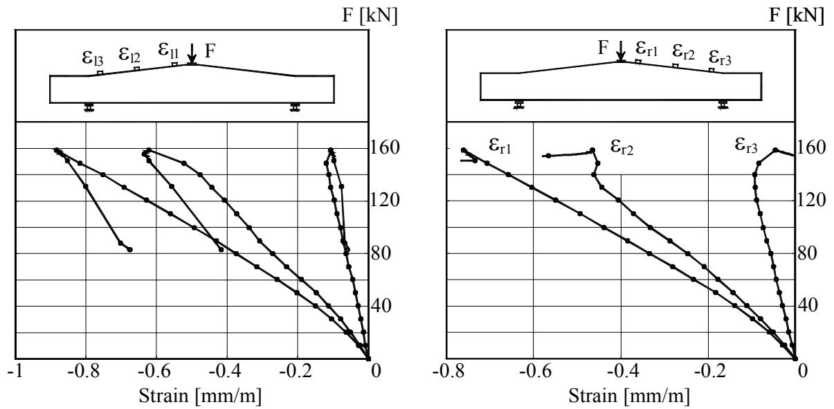
Figure B.3K1.5-The Load –Strains graph at top surface of beam
