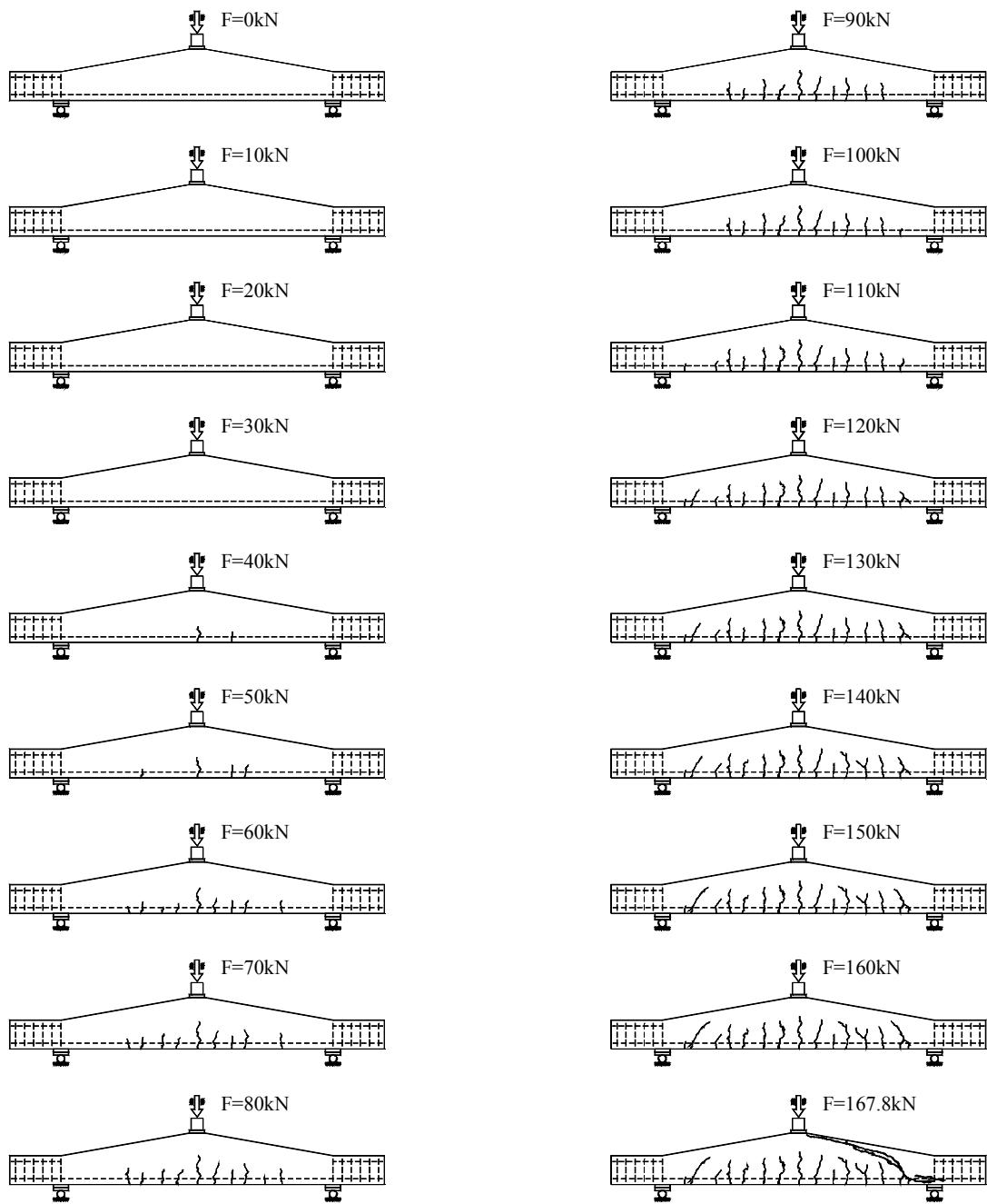
Figure B.4K2.7- Crack propagation of beam 4K2 after each load step.
