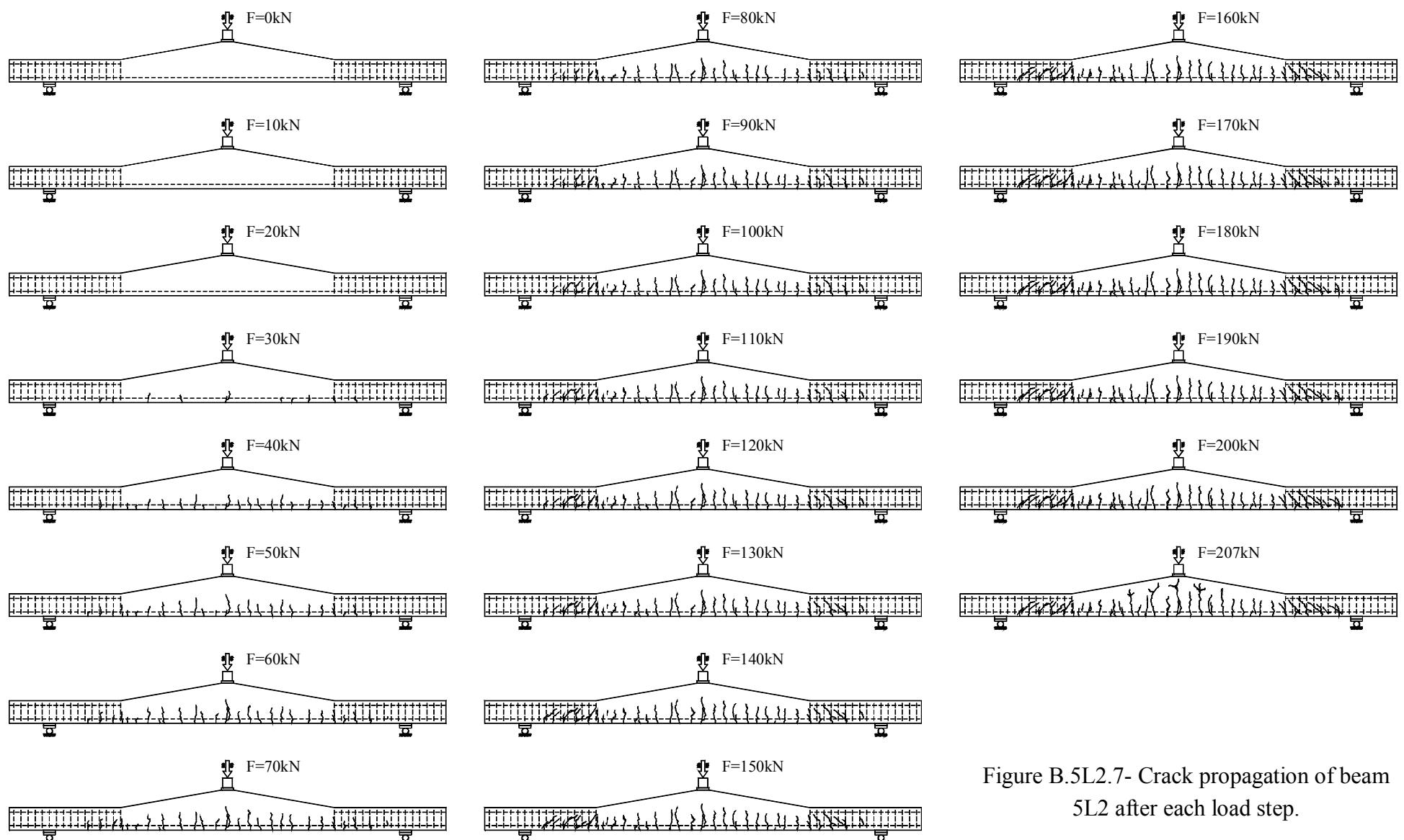
Figure B.5L2.7- Crack propagation of beam 5L2 after each load step.
