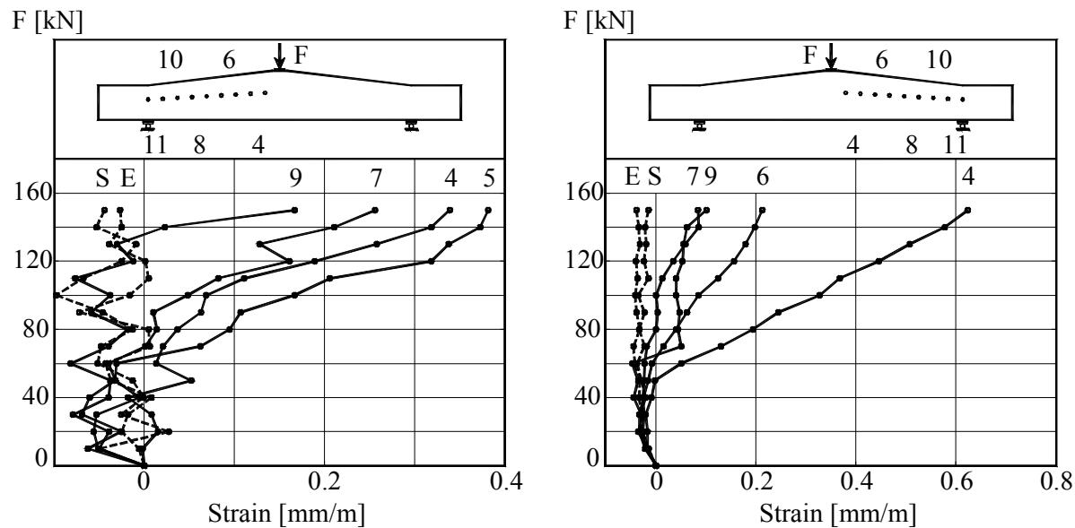
Figure B.3K2.6- The Load –Strains graph at mid-depth of beam
