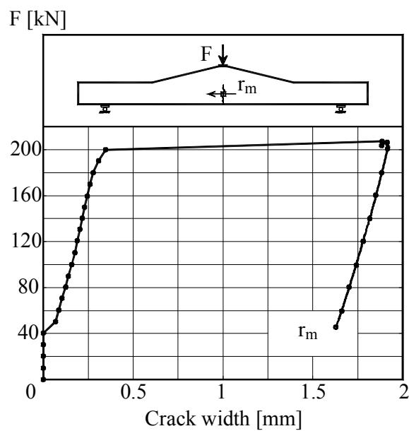
Figure B.5L2.4-The load – crack width graph
