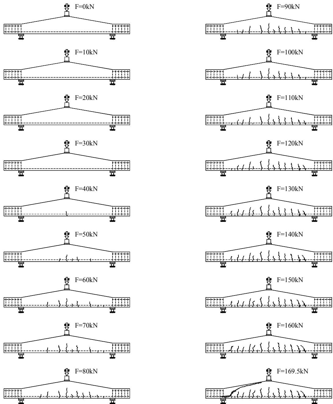
Figure B.4K1.7- Crack propagation of beam 4K1 after each load step.
