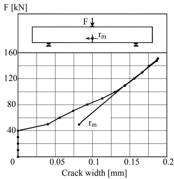
Figure B.1K1.4-The load – crack width graph
