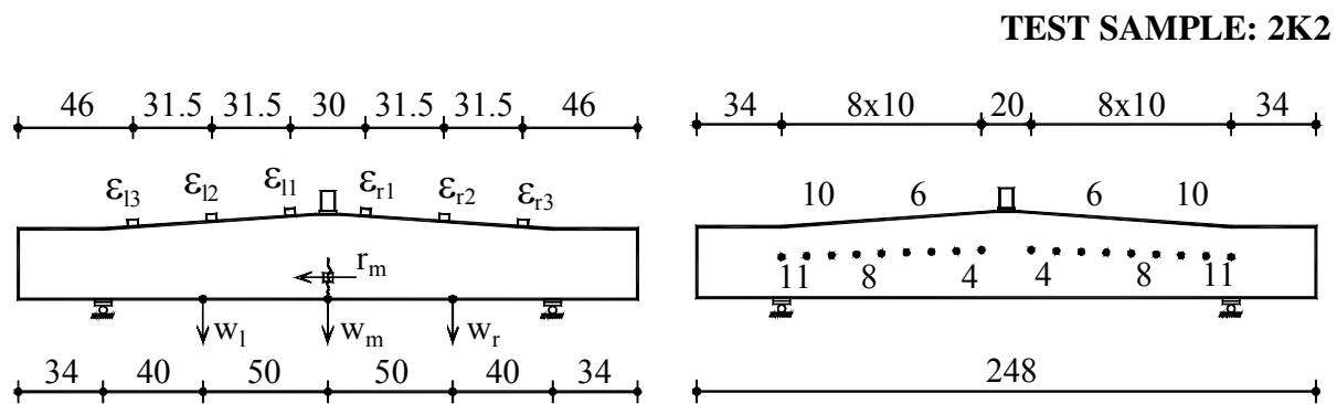
Figure B.2K2.1- The detailed arrangement of the data acquisition system
