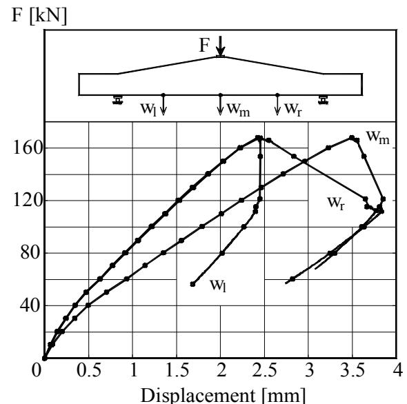
Figure B.4K2.3-The Load – Displacement graph
