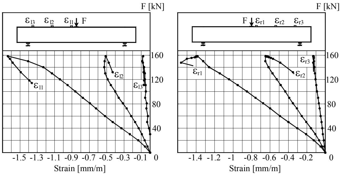
Figure B.1L2.5– The Load –Strains graph at top surface of beam
