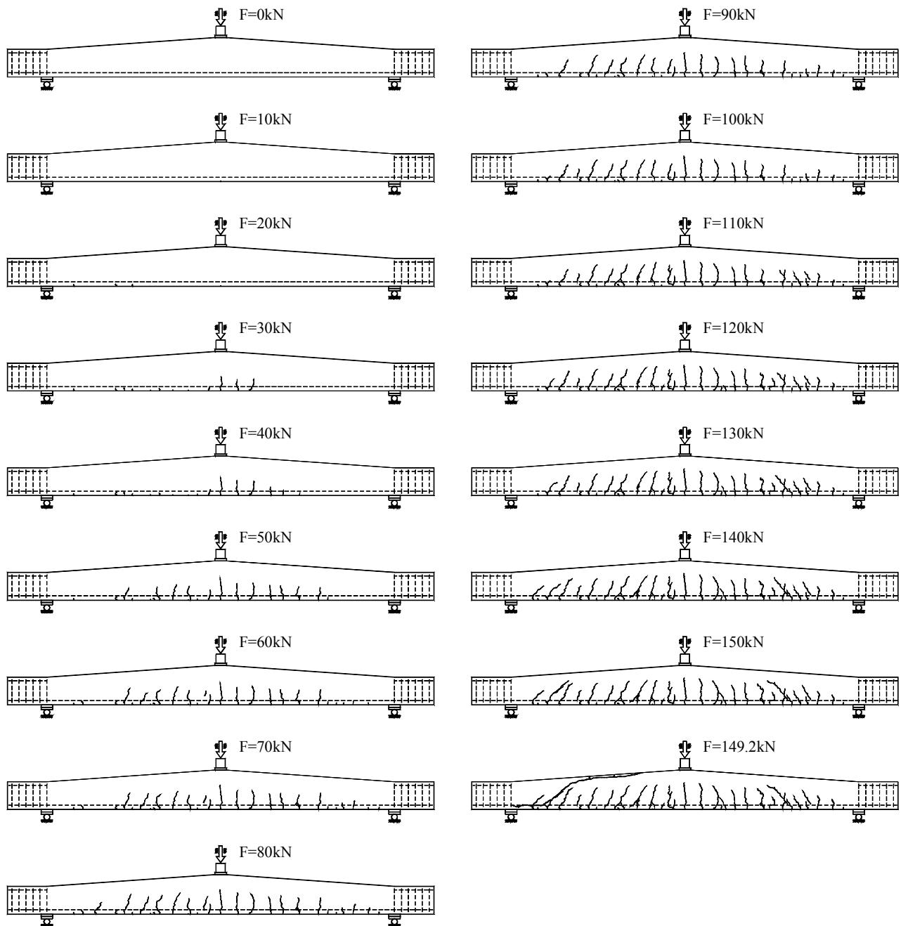
Figure B.2L2.7– Crack propagation of beam 2L2 after each load step.
