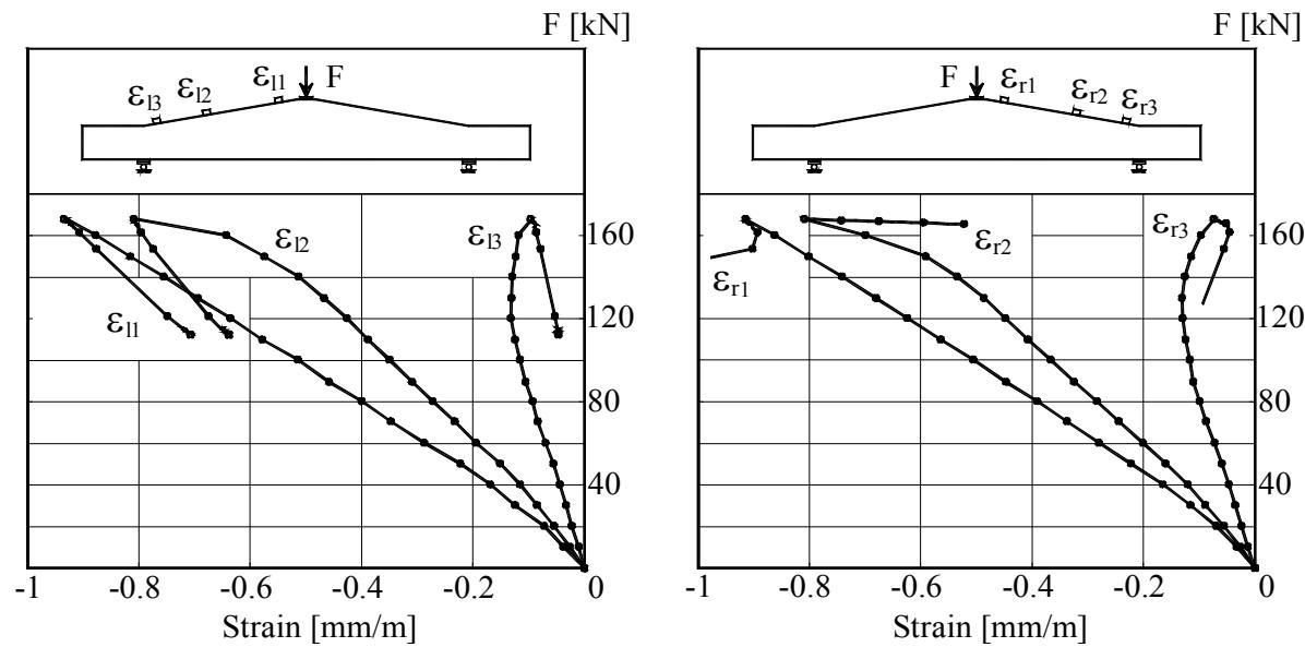
Figure B.4K2.5-The Load –Strains graph at top surface of beam
