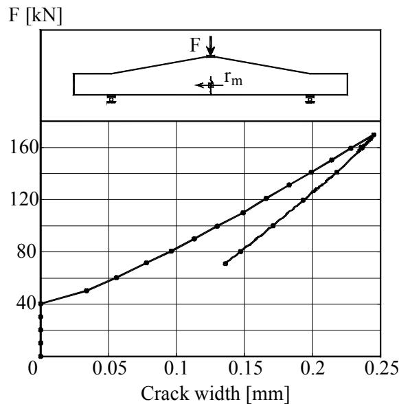
Figure B.4K1.4-The load – crack width graph
