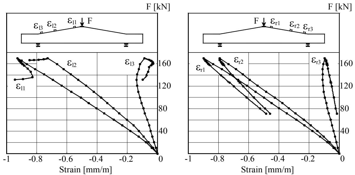
Figure B.4K1.5-The Load –Strains graph at top surface of beam
