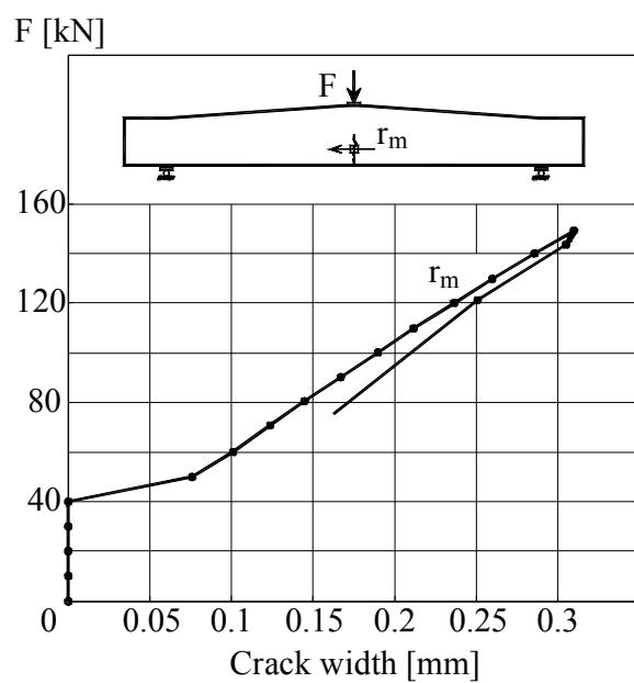
Figure B.2L2.4--The load – crack width graph
