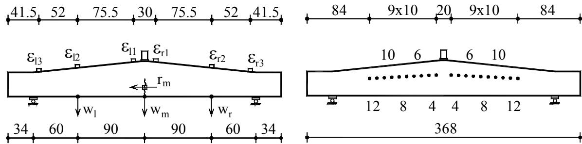
Figure B.3L1.1– The detailed arrangement of the data acquisition system
