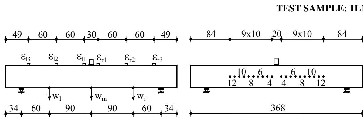
Figure B.1L1.1- The detailed arrangement of the data acquisition system
