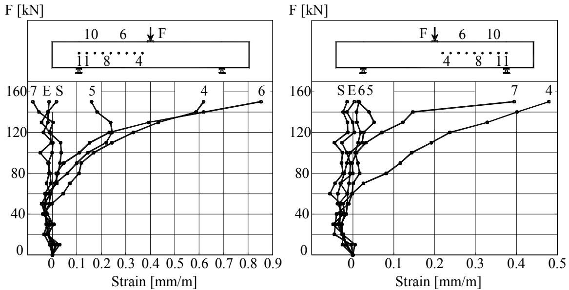
Figure B.1K1.6- The Load –Strains graph at mid-depth of beam
