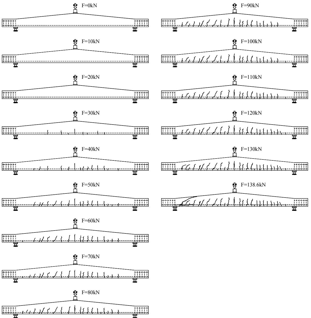
Figure B.3L2.7- Crack propagation of beam 3L2 after each load step.
