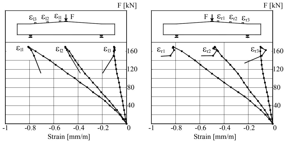
Figure B.2K2.5-The Load –Strains graph at top surface of beam
