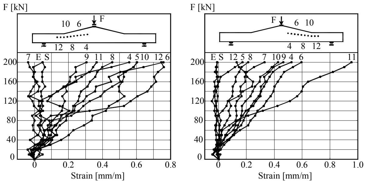
Figure B.5L1.6- The Load –Strains graph at mid-depth of beam
