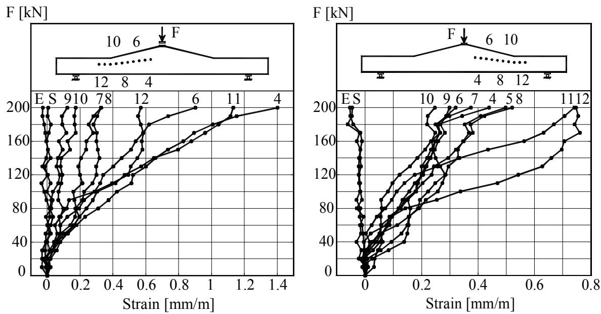
Figure B.5L2.6- The Load –Strains graph at mid-depth of beam
