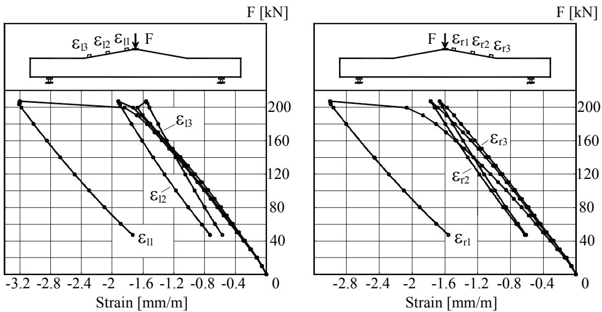
Figure B.4L2.5-The Load –Strains graph at top surface of beam
