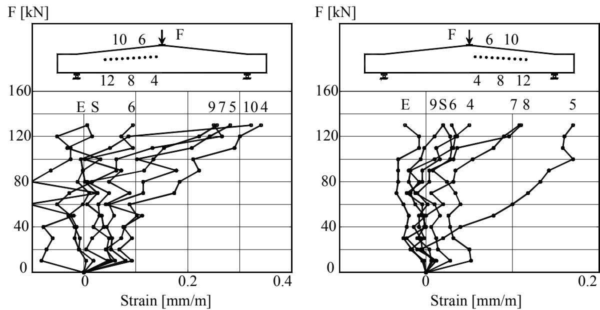
Figure B.3L2.6- The Load –Strains graph at mid-depth of beam
