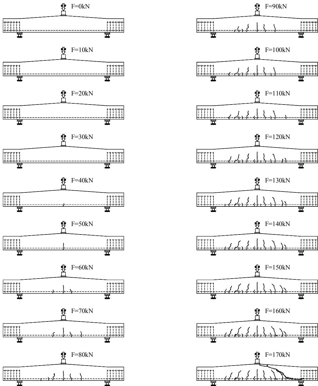
Figure B.2K2.7- Crack propagation of beam 2K2 after each load step.
