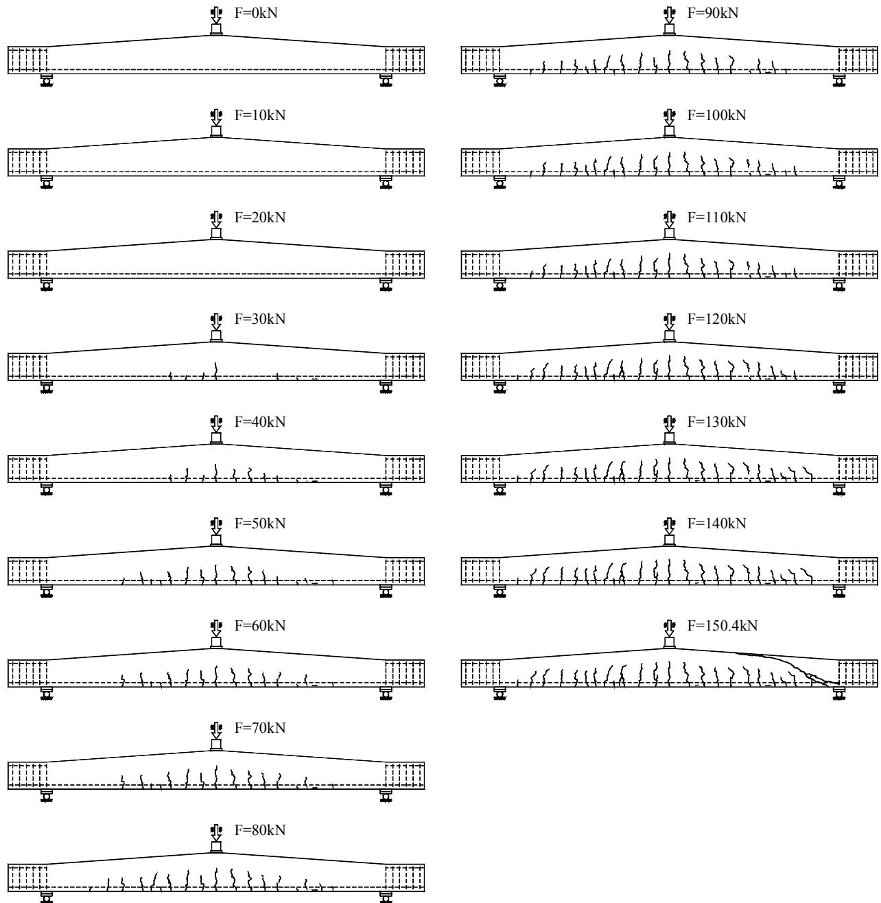
Figure B.2L1.7– Crack propagation of beam 2L1 after each load step.
