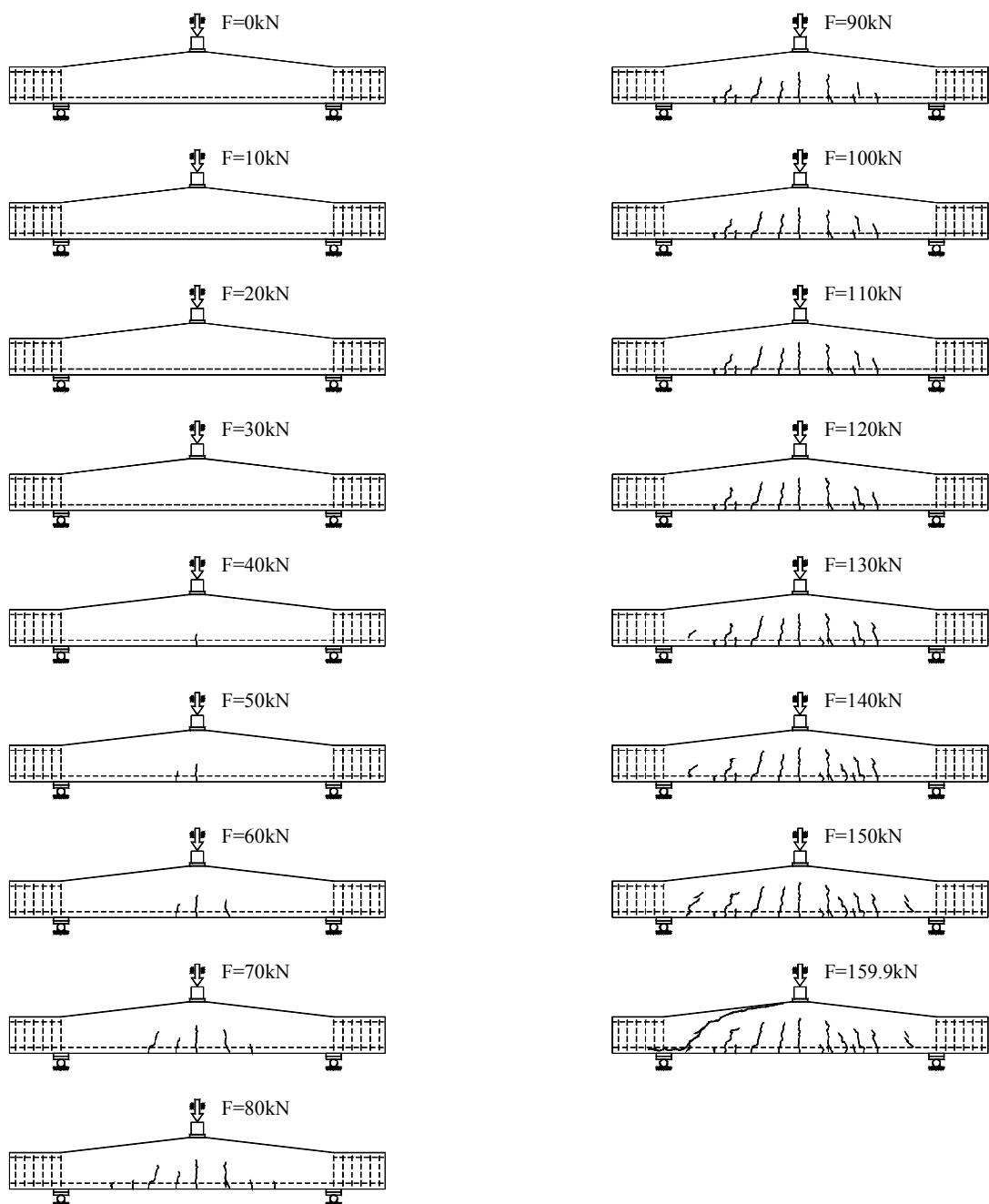
Figure B.3K2.7- Crack propagation of beam 3K2 after each load step.
