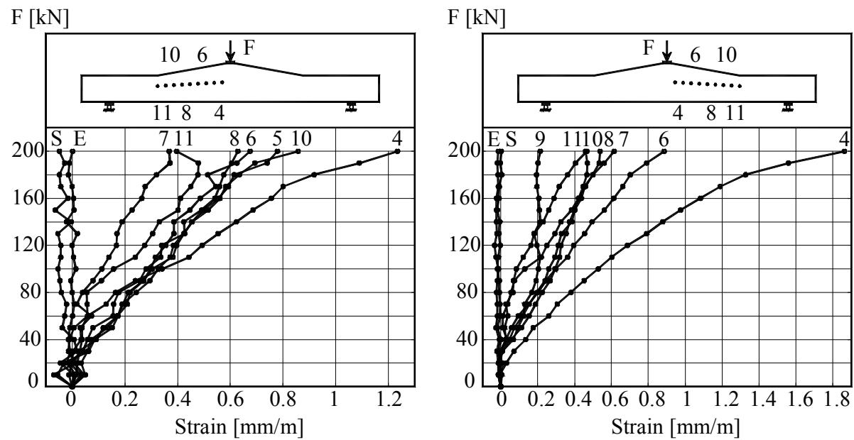
Figure B.4L2.6- The Load –Strains graph at mid-depth of beam
