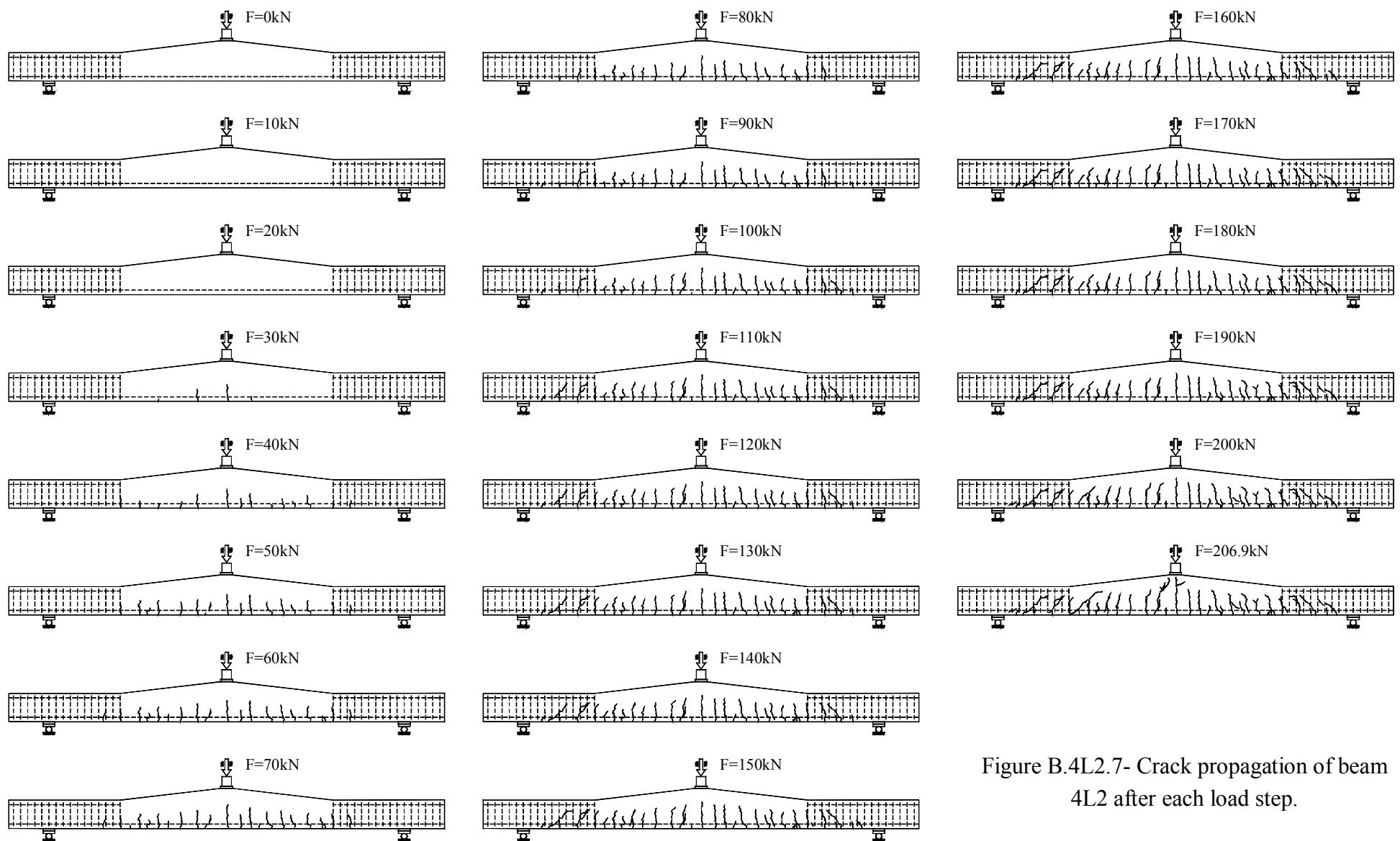
Figure B.4L2.7- Crack propagation of beam 4L2 after each load step.
