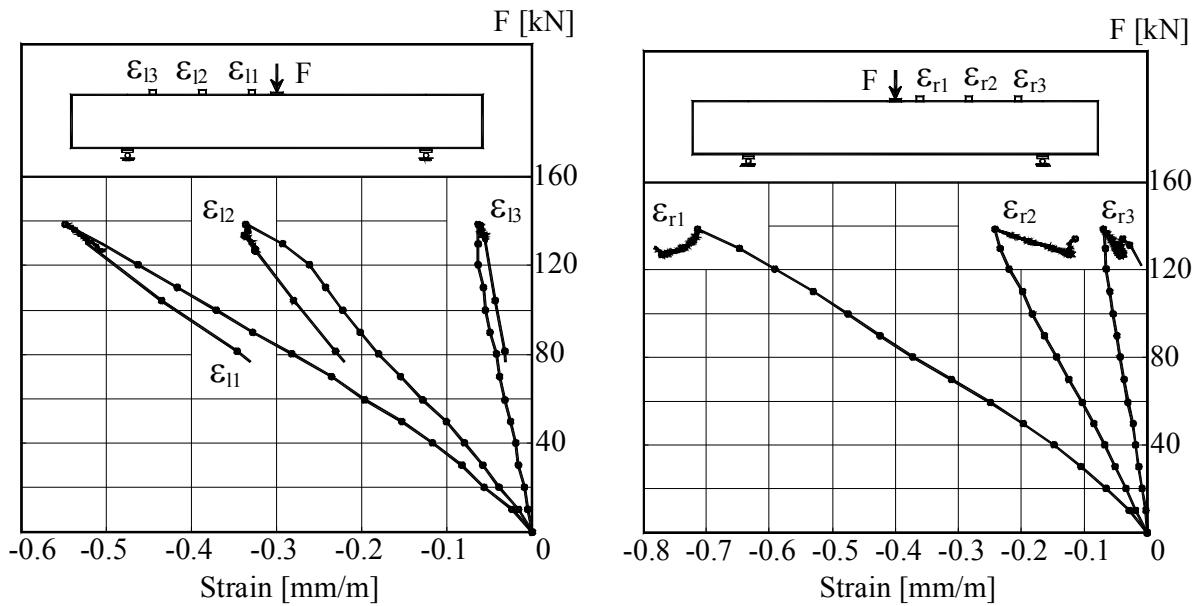
Figure B.1K2.5-The Load –Strains graph at top surface of beam
