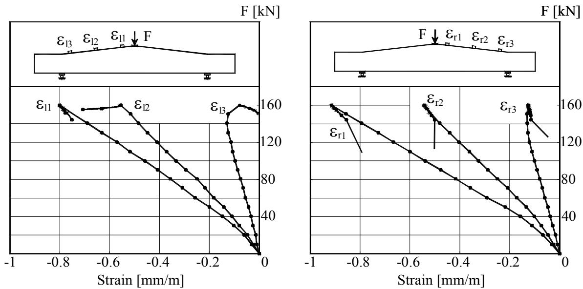
Figure B.3K2.5-The Load –Strains graph at top surface of beam
