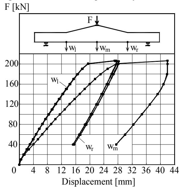
Figure B.5L1.3-The Load – Displacement graph
