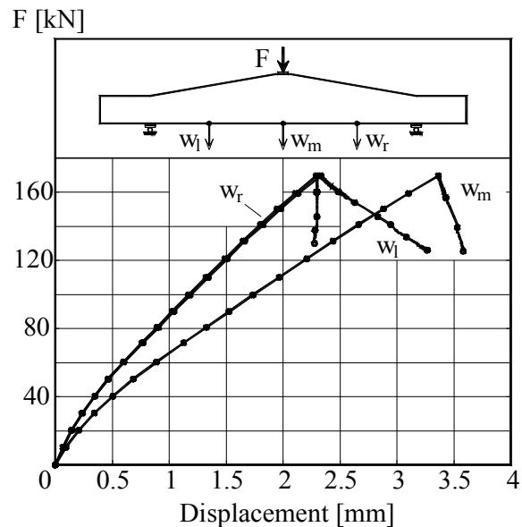
Figure B.4K1.3-The Load – Displacement graph
