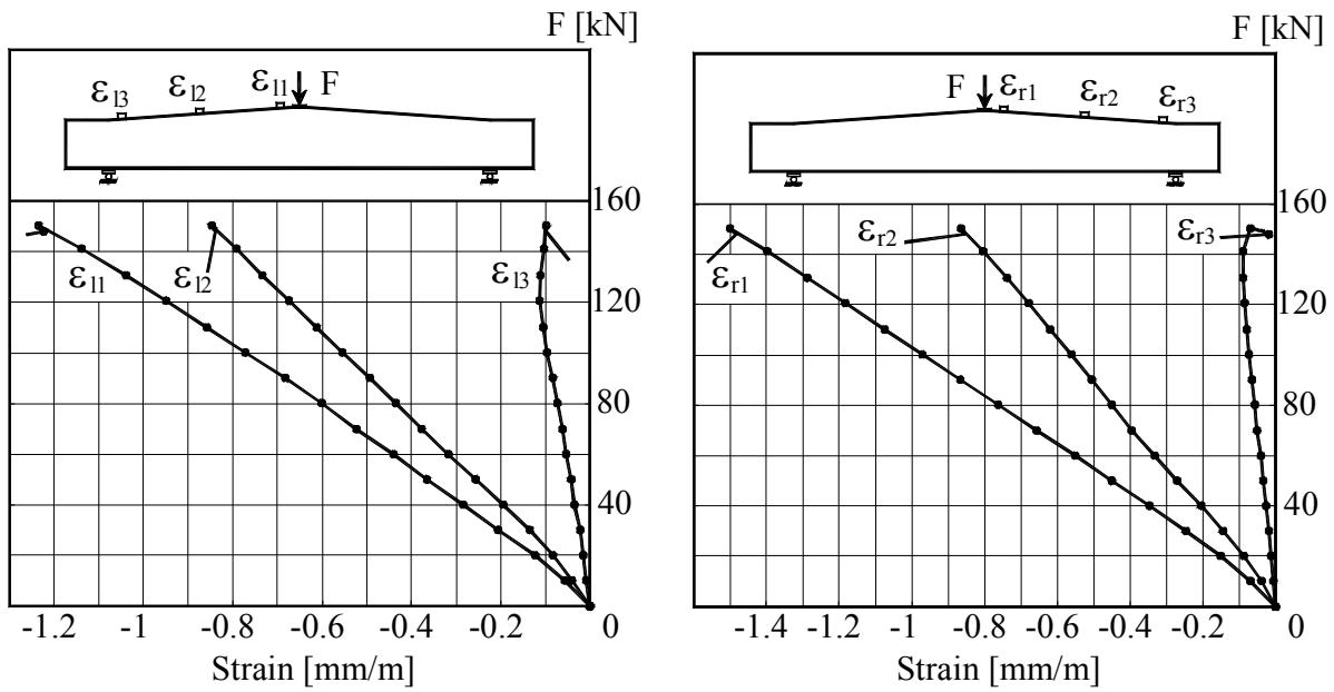
Figure B.2L1.5– The Load –Strains graph at top surface of beam
