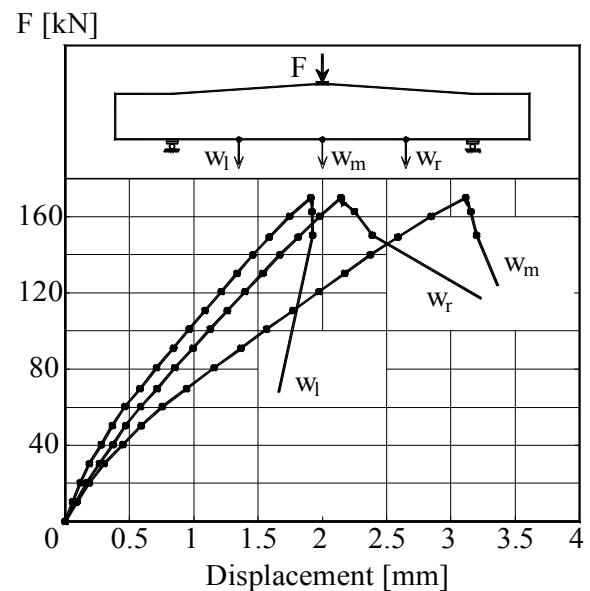
Figure B.2K2.3-The Load – Displacement graph
