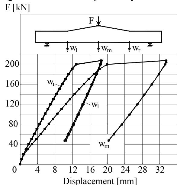
Figure B.4L2.3-The Load – Displacement graph
