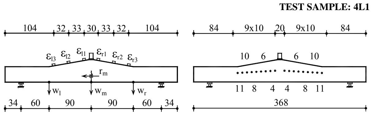
Figure B.4L1.1- The detailed arrangement of the data acquisition system
