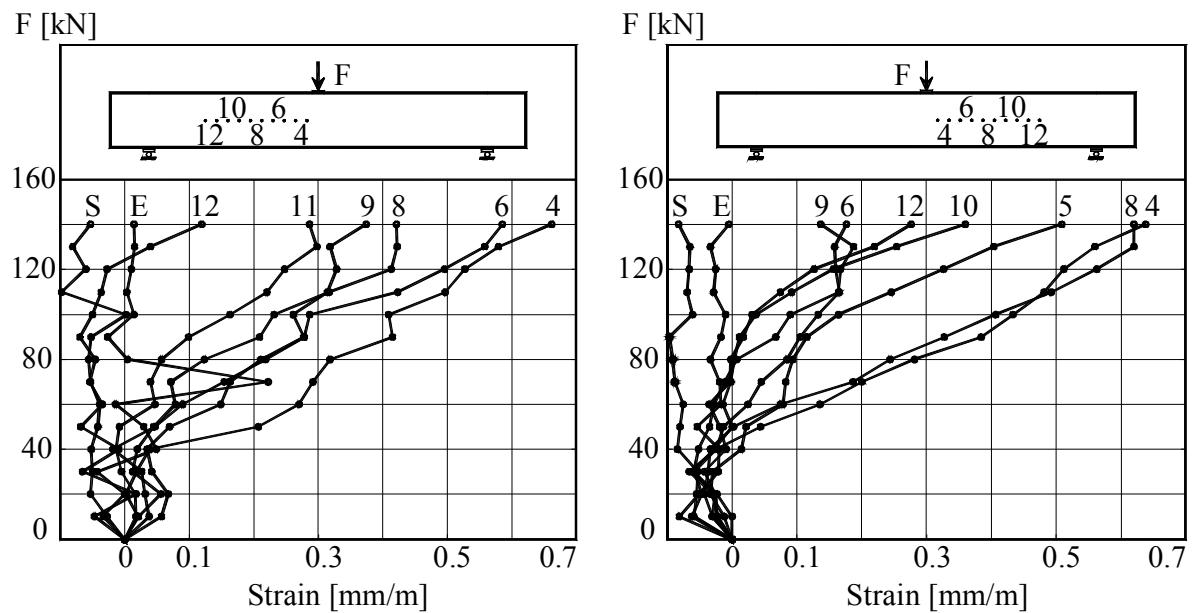
Figure B.1L1.5– The Load – Strains graph at mid-depth of beam
