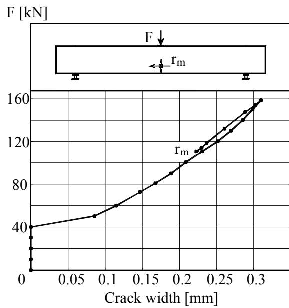
Figure B.1L2.4– The load – crack width graph
