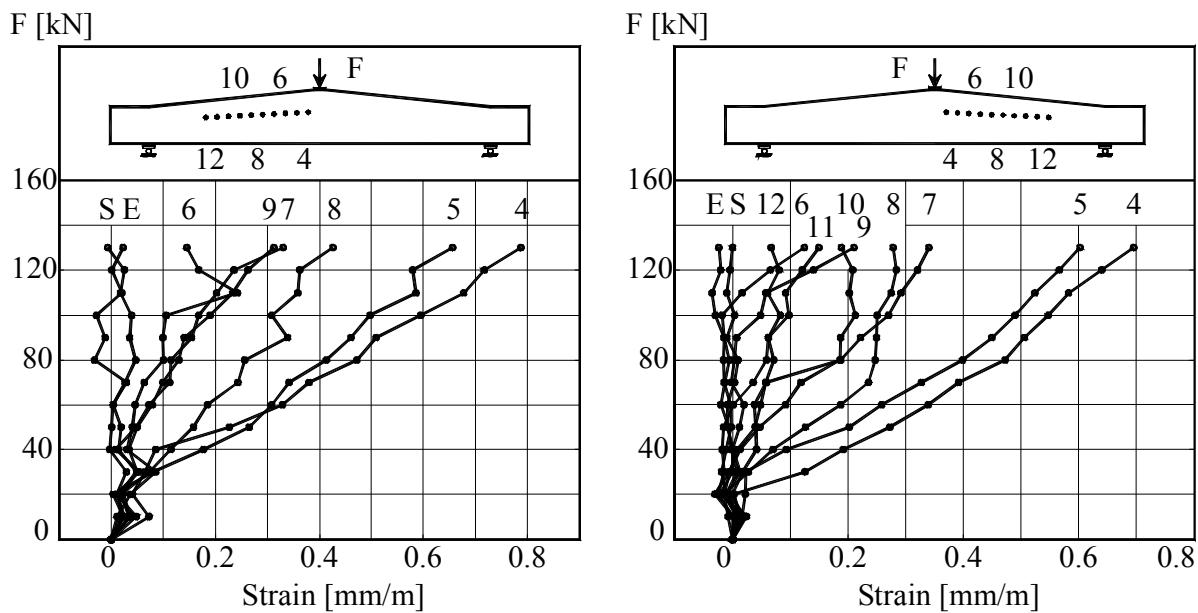
Figure B.3L1.6– The Load –Strains graph at mid-depth of beam
