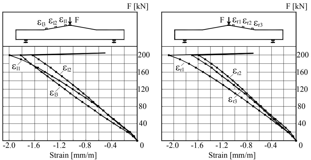
Figure B.4L1.5-The Load –Strains graph at top surface of beam
