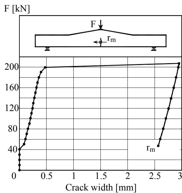
Figure B.4L2.4-The load – crack width graph
