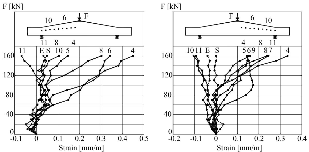
Figure B.4K1.6- The Load –Strains graph at mid-depth of beam
