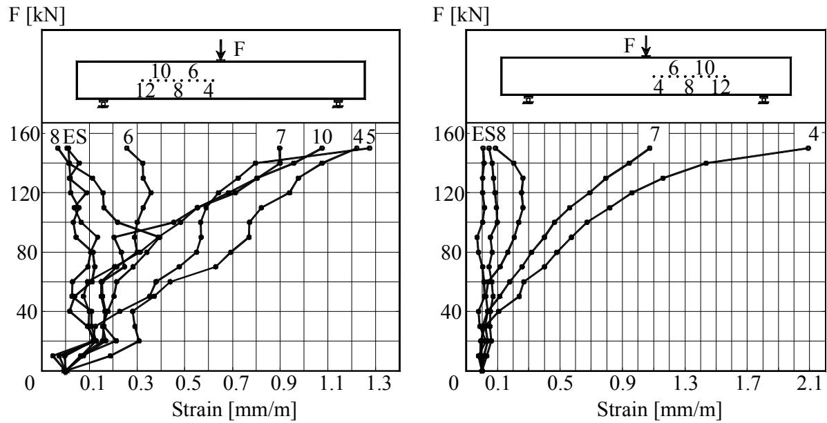
Figure B.1L2.6– The Load –Strains graph at mid-depth of beam
