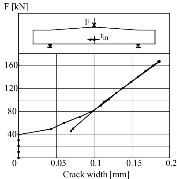
Figure B.2K1.4-The load – crack width graph
