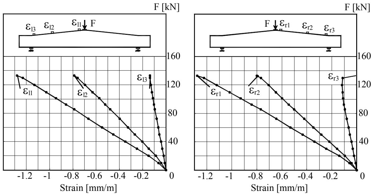
Figure B.3L1.5– The Load –Strains graph at top surface of beam
