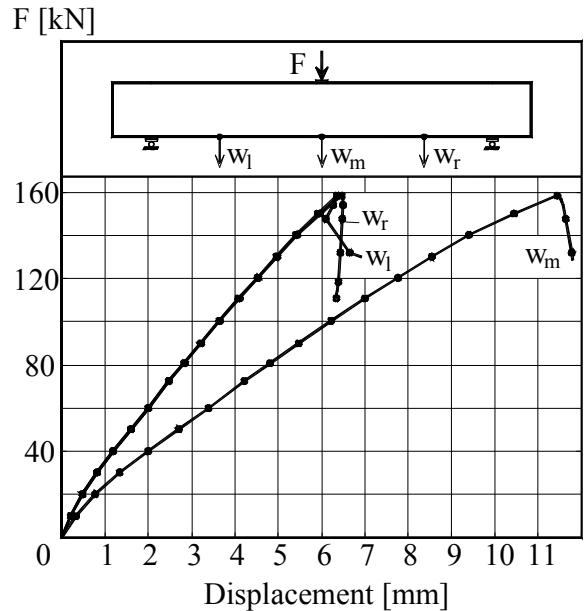
Figure B.1L2.3– The Load – Displacement graph
