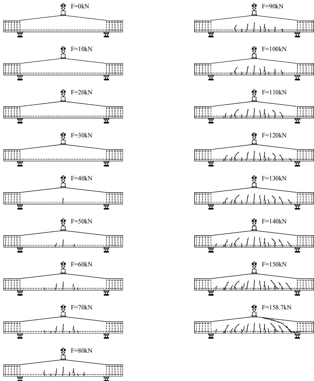
Figure B.3K1.7- Crack propagation of beam 3K1 after each load step.
