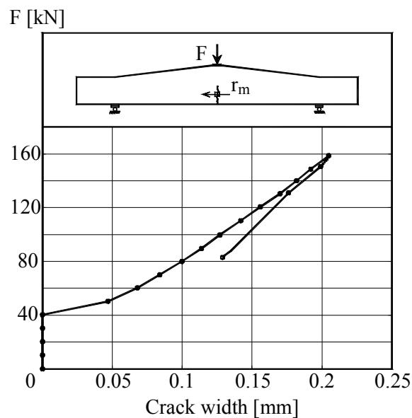
Figure B.3K1.4-The load – crack width graph
