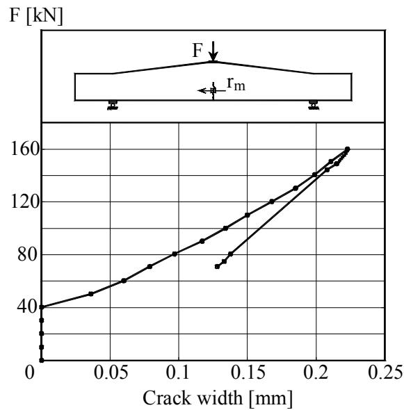
Figure B.3K2.4-The load – crack width graph
