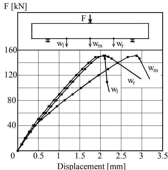
Figure B.1K1.3-The Load – Displacement graph
