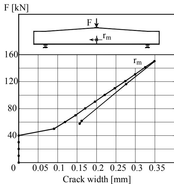
Figure B.2L1.4 – The load – crack width graph
