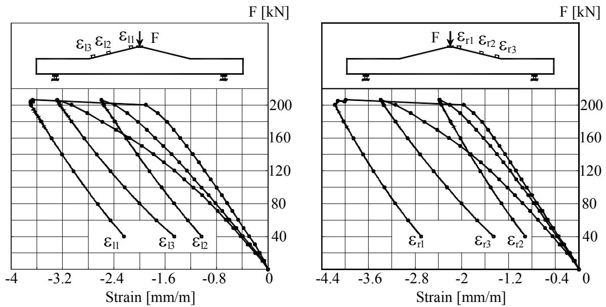
Figure B.5L1.5-The Load –Strains graph at top surface of beam
