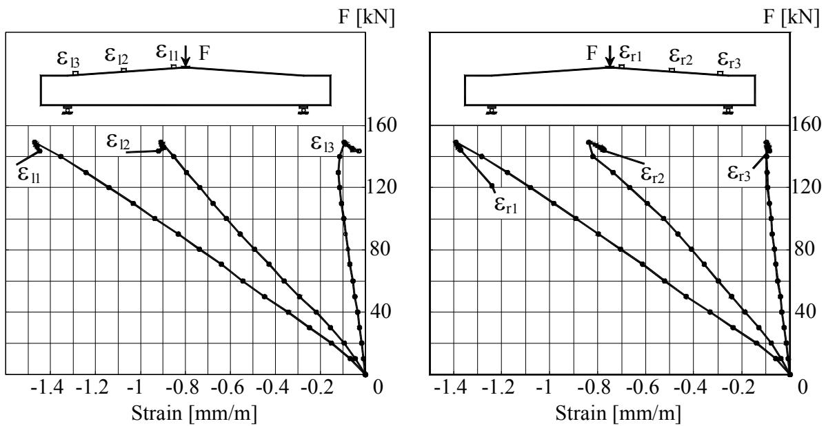
Figure B. 2L2.5 – The Load –Strains graph at top surface of beam
