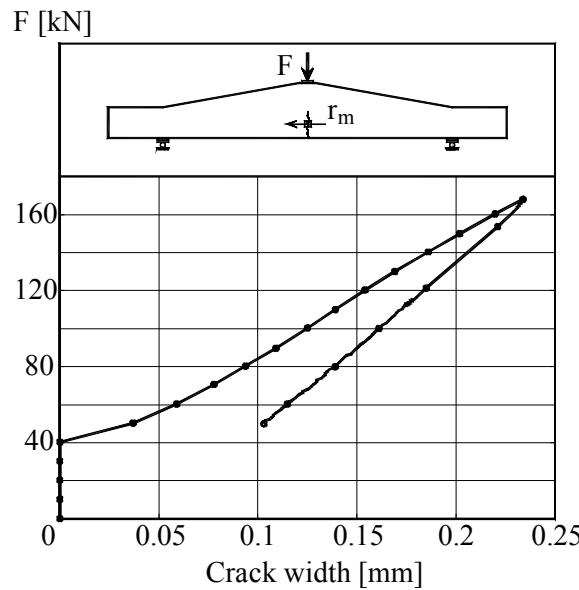
Figure B.4K2.4-The load – crack width graph
