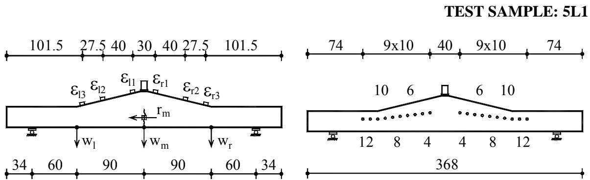
Figure B.5L1.1- The detailed arrangement of the data acquisition system
