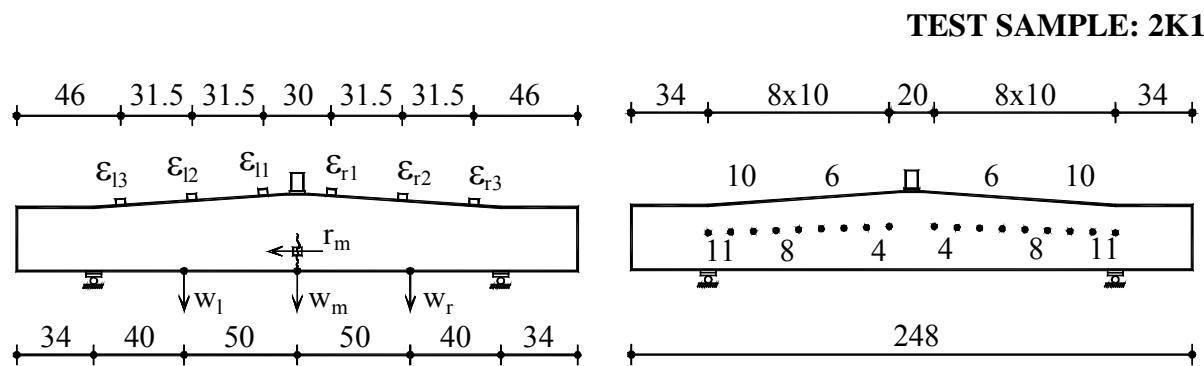
Figure B.2K1.1- The detailed arrangement of the data acquisition system
