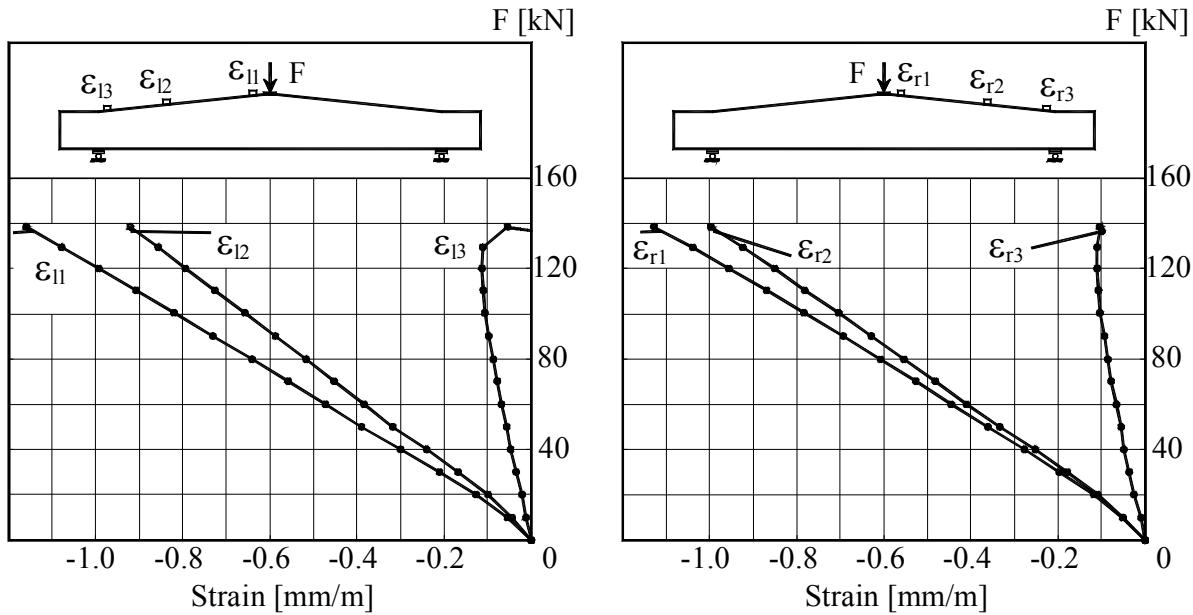
Figure B.3L2.5-The Load –Strains graph at top surface of beam
