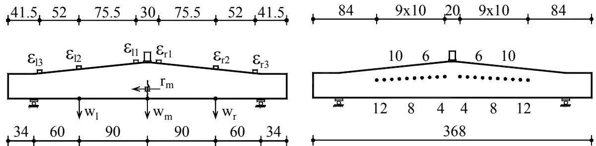
Figure B.3L2.1- The detailed arrangement of the data acquisition system
