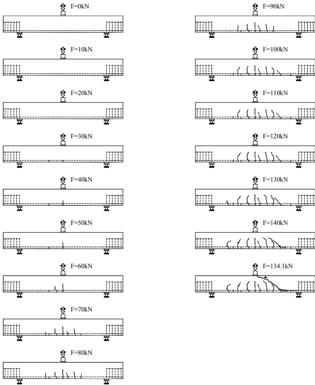
Figure B.1K2.7- Crack propagation of beam 1K2 after each load step.
