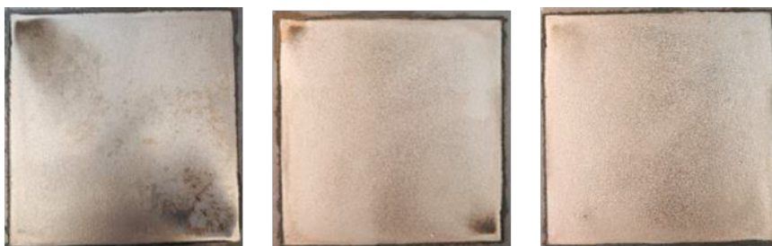
Fig. 5 Coating of flat sheets; from left to right reduction of the pump speed of the peristaltic pump (left: 5.9 l/min; middle: 4.4 l/min; right: 2.8 l/min).
