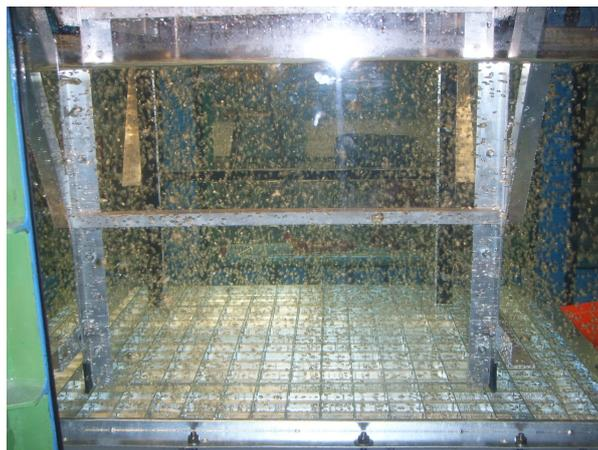
Figure 3: Air bubbles ascending from pressure tank membrane between model guiding.
