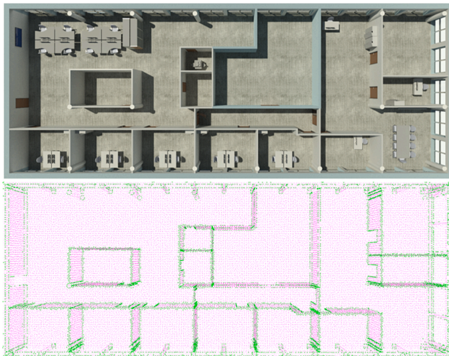
Fig. 8. Extracted edge and planar feature points of the BIM model of the indoor office environment.
