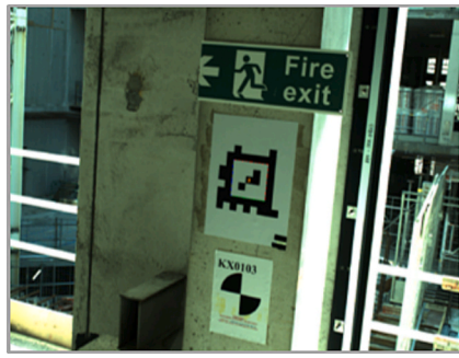
Fig. 9. AprilTags visible in the color camera images of the ConSLAM dataset are placed in the BIM model to obtain the transformation from map frame to BIM model frame.
