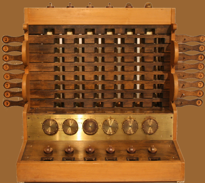
The Schickard machine is a non-programmable calculating machine for integers invented by Wilhelm Schickard (1592-1646).
