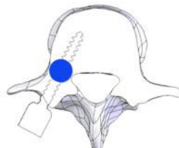
(C) Cement concentrated towards the screw head
