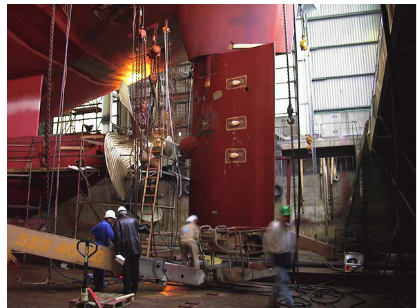
Figure 9. Rudder and propeller of the validation case of the full scale vessel during construction. Source: Image archive M-06, TUHH.
