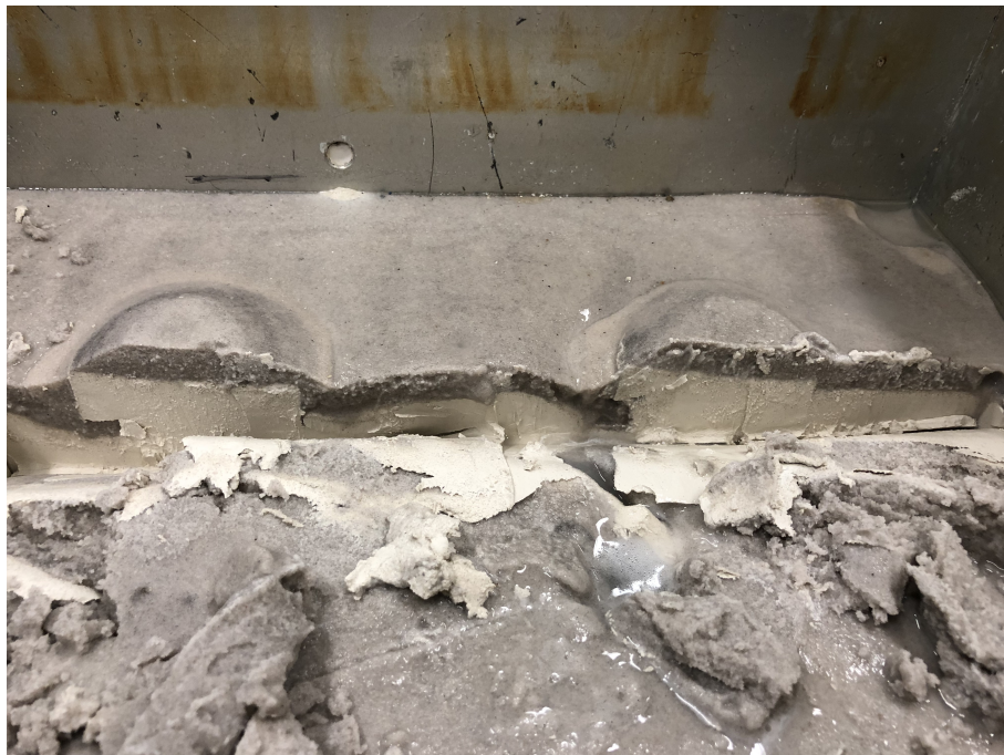
Figure B.20: Cross-section of two rapid extraction sites in the sand over clay sample.
