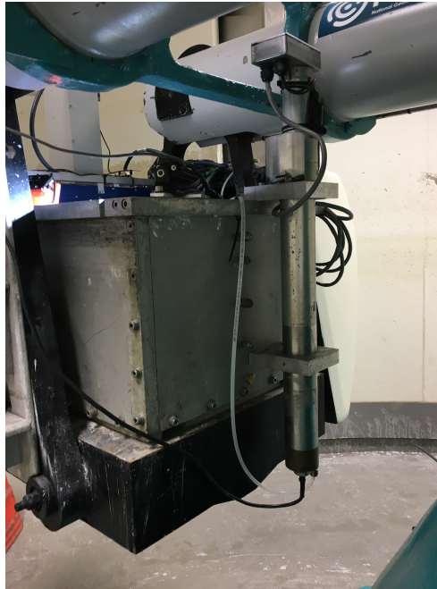
Figure B.8: Syringe pump mounted at the backside of the strong box.
