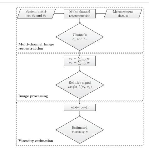
**Figure 3.** The diagram summarizes all processing steps of the viscosity estimation. First, the measurement  $\hat{u}$  of a sample is multichannel reconstructed using the system matrices  $S_1$  and  $S_7$ . Second, the multi-channel image is processed to obtain the relative signal weight. At last, the viscosity is estimated by inverting a data driven calibration curve.
