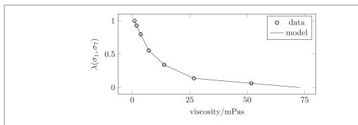
**Figure 4.** A quarter of the data sets of M1 to M7 with  $M_{avg} = 100$  is used to obtain the calibration points shown above. These points are used to create a piece wise linear model, which can be inverted to estimate the viscosity of the remaining data sets.
