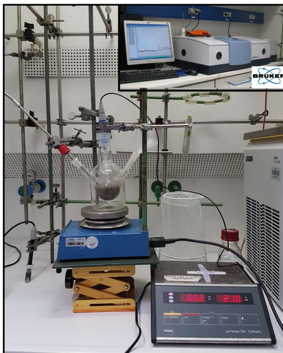
Figure A.2.4: Experimental setup for ATR-FT-MIR inline measurements.
