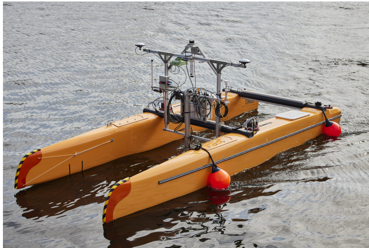
Figure 4: SeaDragon USV, catamaran used for validating the Guidance module
