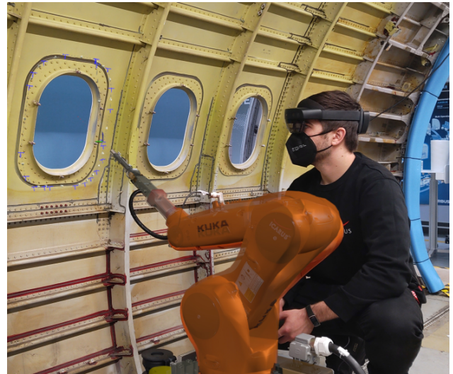
FIG 5. AR-assisted robot programming in aircraft fuselage manufacturing.
