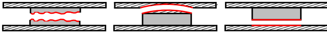
Figure 2.10: Failure modes of a bonded joints: a) Cohesive failure in the adhesive layer; b) Cohesive failure in the adherend; c) Adhesive failure.
