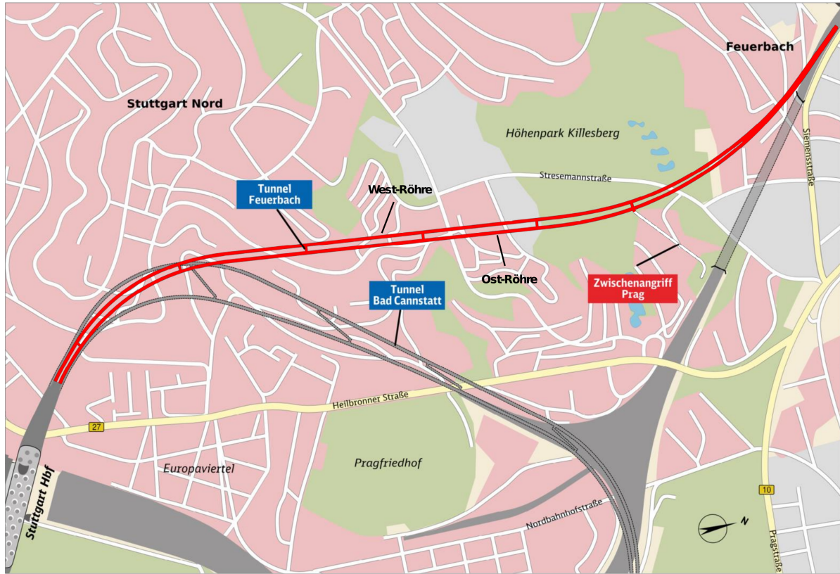
Figure 5.3: The tunnel Feuerbach connects the main station Stuttgart with the station Feuerbach. The tunnel consists of two parallel tubes, which are connected with several connection buildings. Construction equipment enters the tunnel construction site at Zwischenangriff Prag. Source DB Projekt Stuttgart-Ulm (2019).
