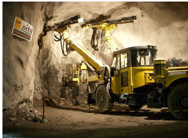
Figure 5.9: Exemplary picture of drilling jumbo. The drilling jumbo produces the boreholes, which are later being injected with chemical grouting material. Picture by Ellgaard (2009).
