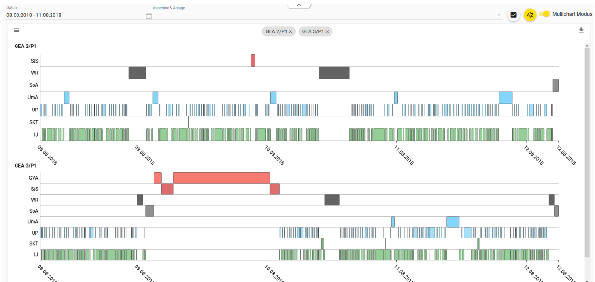
Figure 5.13: Screenshot of the visualization of processes with eguana-SCALES, eguana (2019). Each of the two diagrams shows the documentation of one pump’s activities during the project. Depicted are five days during which pump GEA 2/P1 (top) performs seven and pump GEA 3/P1 (bottom) eight different types of processes.
