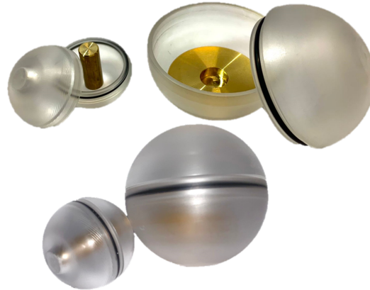
Figure 3. LSP design for tracking of flow-following capabilities in a vessel used in this study. With 25 mm equatorial LP and respective cylindrical brass insert ( top left ). The 40 mm off-center LP with respective brass insert shifting the CoM ( top right ). Closed 25 mm equatorial and 40 mm off-center LP ( bottom ).
