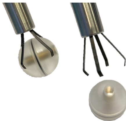
Figure 6. Clasp and release of a 25 mm LP.
