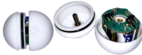
Figure 1. LSP design by [15] used as inspiration for this work. With the LSP almost shut ( left ), the threaded rod visible in the upper half shell ( center ), and the internal sensors and circuit boards as well as power source ( right ).
