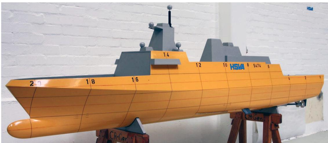
Figure 4.5.: ship model used for model tests
