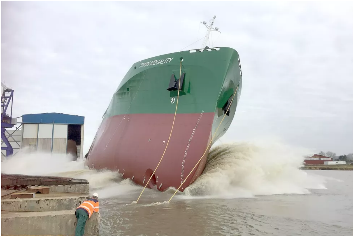
Figure 1.1.: sideways launching process of Thun Equality [66]
