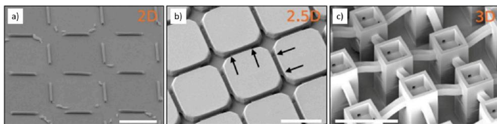
Figure 34. Scanning electron microscopy (SEM) images of devices utilizing spatial restriction in 2D, 2.5D, and 3D during cell culturing to control neuronal growth. (a) 2D pathways are defined by rolled-up GaAs/InGaAs microtubes. (b) Cavities and grooves with steps (arrows) are prepared by photolithography and reactive ion etching, defining 2.5D pathways for neuronal guidance. (c) Direct laser writing (DLW)-prepared scaffold structure with towerlike cavities connected by free-standing tunnels. The scale bars represent 50 \mu\text{m} . Original images are modified with permission from (a) Bausch et al. 804 Copyright 2013 AIP Publishing; (b) Fendler et al. 105 Copyright 2019 Wiley VCH Verlag; (c) Fendler et al. 112 Copyright 2020 Royal Society of Chemistry.
