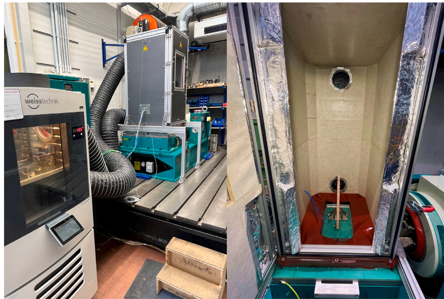
Fig. 2. The environmental chamber at the electrodynamic shaker.
