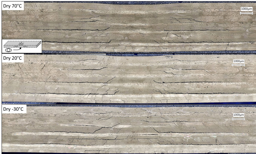
Figure 4.52: Images of representative microscopic cross sections of the impacted area (central cut) for three impact temperatures in dry conditions.
