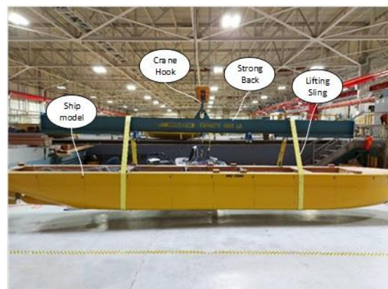
Figure 4-Hammer test on the scaled model structure
