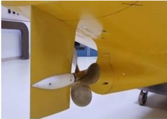
Figure 2- Propeller mounted aftship of the model
