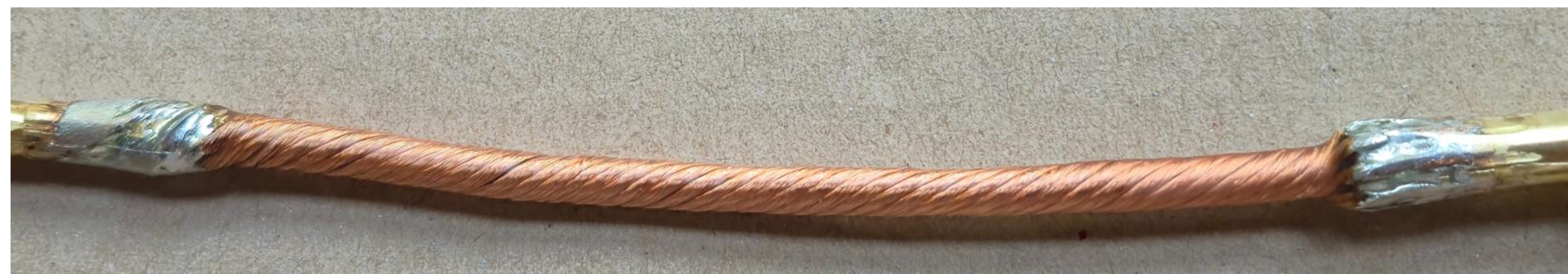
Prototype of a litz wire hollow conductor with a thermoset matrix for pressure testing (result: pressure tight up to the maximum tested pressure of 4.8 bar)
