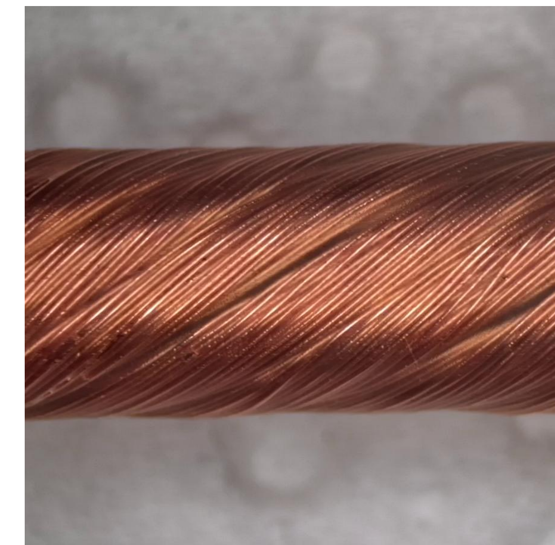
Outside surface and cross-section of hollow conductor
