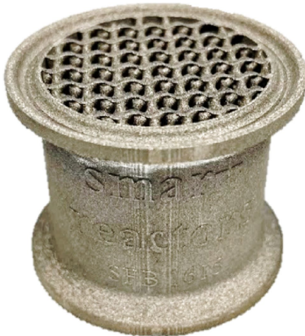
Fig. 16 An additively manufactured module featuring a TPMS structure, directly connected to the wall, used for the pressure drop study
