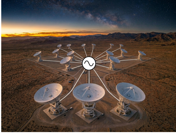
(a) Illustration of an array of radio telescopes with star-topology RF network.
