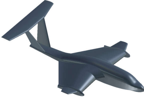
Fig 3: The WIGS shape of CFD investigated
