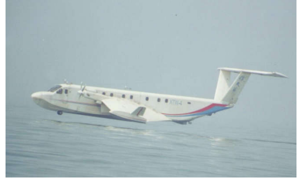
Fig 4: The WIG vehicle of XTW-4 in trial
