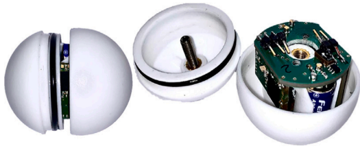
Fig. 2. Depiction of the LSP design by Buntkiel et al. [29] with the two connected half-shells (left), the top half-shell with its threaded rod (center), and the bottom half-shell including the electronics (right) [33].
