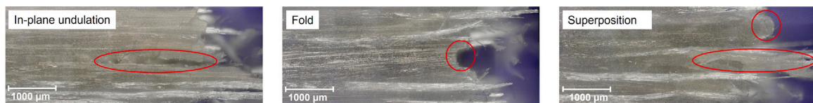
Fig. 12. Damage of representative fatigue specimens after failure.
