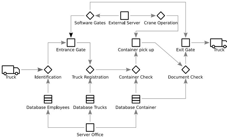
Figure 2: Important components for container pick up
