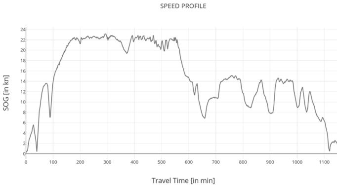
Figure 4: Average speed profile of trips from Rotterdam to Hamburg
