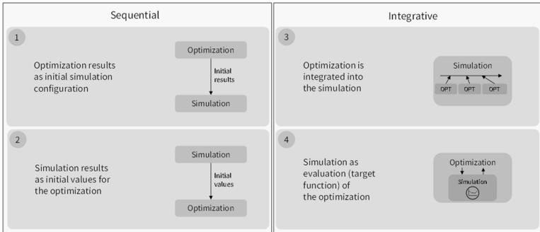
Figure 3: Types of linking simulation and optimization
