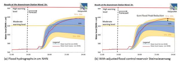
Fig. 3. (a) Quantile plot of the flood hydrographs of 10 ensembles member runs in cm NHN of the rainfall event 28 August 2016 at the station Niendorfer Str.. Flood hydrographs based on radar measurements (blue) and water level measurements (red). (b) Plotted flood hydrograph results of the adjusted FCR Steinwiesenweg illustrating the reduction of 6cm in peak water level.
