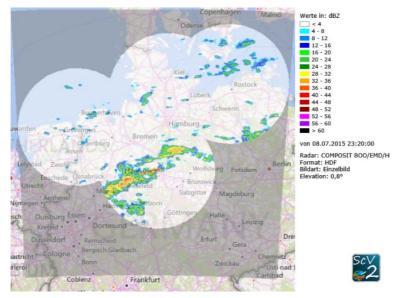
Figure 1. Operational North German composite from four radars Boostedt, Emden, Hannover, Rostock in dBZ
