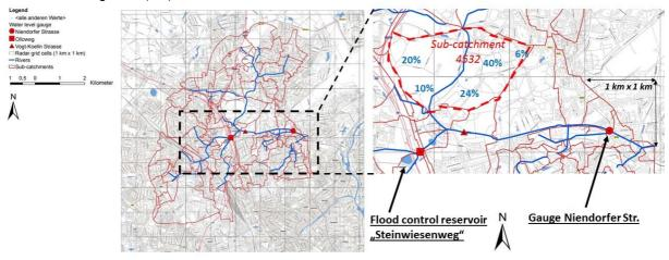
Fig. 2. Map of the Kollau catchment (33.6 km<sup>2</sup>), location of water level gauges, illustration of the intersection of precipitation data with hydrological elements and the location of the FCR 'Steinwiesenweg'.
