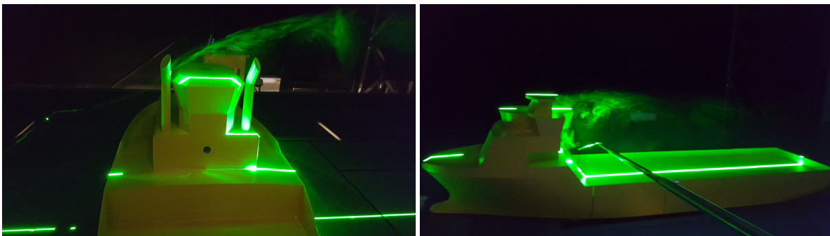
Figure 4.13: Visualization of turbulent flow at the tug's funnel (left), wake behind the deck house of the OSV (right)
