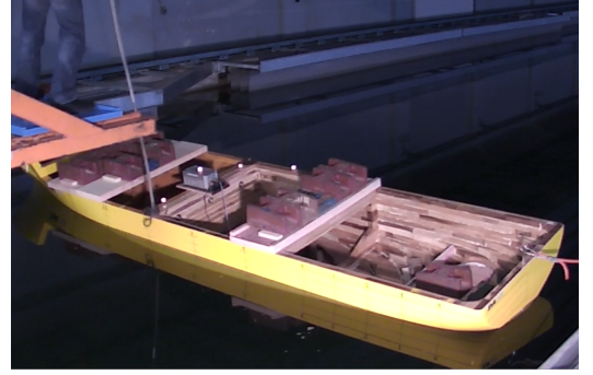
Figure 3.3: Experimental and numerical decay test \varphi_0 = 9.64^\circ
