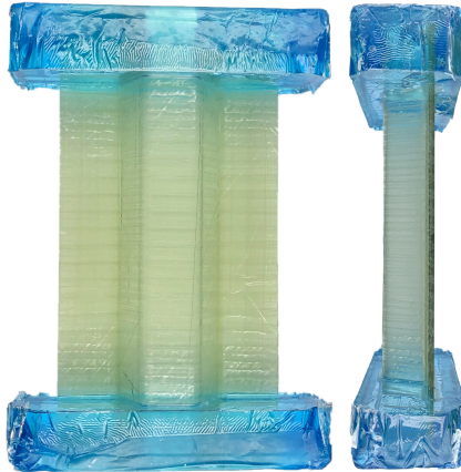
Figure 4.3: Photographs of reference stringer specimen without integrated film sensors
