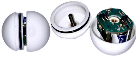
Fig. 2. Depiction of the LSP design by Buntkiel et al. [29] with the two connected half-shells (left), the top half-shell with its threaded rod (center), and the bottom half-shell including the electronics (right) [33].
