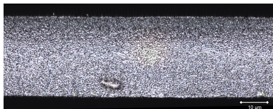
Figure 5.6: Cutting edge of an as-produced sample type C with a thickness of 30 μm create by laser.
