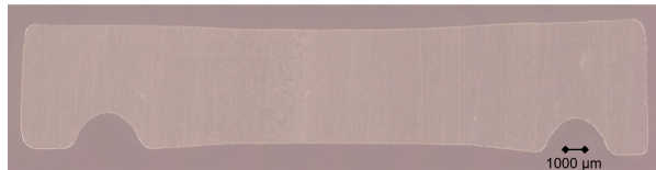
Figure 1: Microscopic image of a punched type A sample with a thickness of 30 μm.
