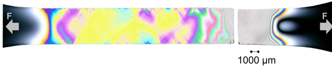
Figure 5.21: Photoelastic image of deformed bulk samples with a thickness of 2000\ \mu\text{m} after creep loading (70 % UTS).
