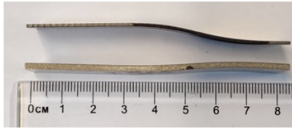
Fig. 4.16: Exemplary 1 mm and 2 mm thick Ti6Al4V LPF treated specimens bidirectionally bent to target shapes from initially flat shape.
