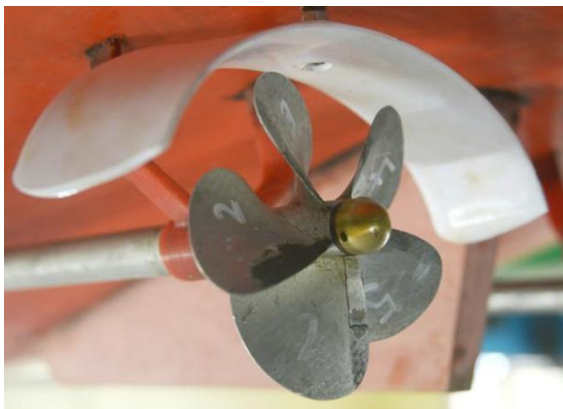
Fig. 16: The partial duct fitted over the propeller during the model self-propulsion tests.
