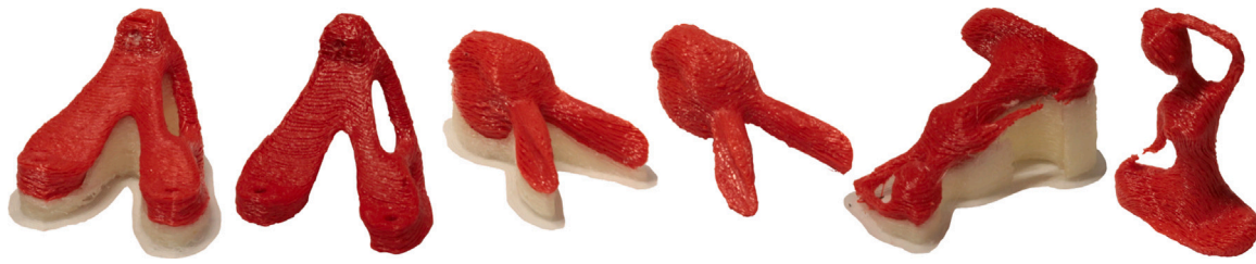
Fig. 10. Results of the physical fabrication using a multi-axis 3D-printer. From left to right with and without support material: Topopt , Bunny , Yoga .
