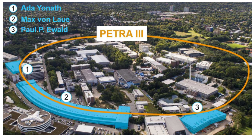
Figure 2.6: Aerial view of the PETRA III storage ring and the three experimental halls at Deutsches Elektronen Synchrotron DESY, Hamburg, Germany. Picture is adopted from [100](modified). Copyright: DESY, Britta Liebaug Illustration, Reimo Schaaf Picture.
