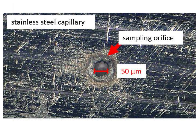
Figure 3.3: Photograph of a sampling orifice laser-drilled in a stainless steel sampling capillary.
