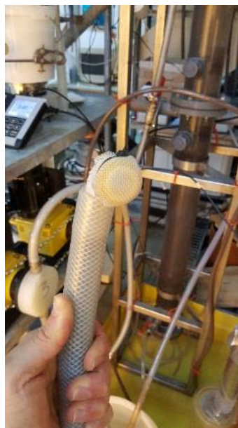
Figure 60. Conditioning of SFBBR-2. Installation of protecting mesh at input line
