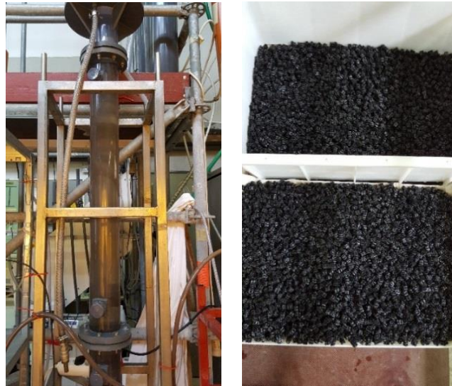
Figure 55. Conditioning of SFBBR-2. Left: Empty column; Right: Carrier material left drying
