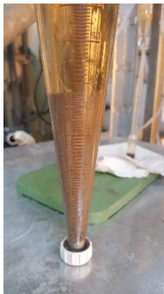
Figure 61. Sludge collected from SFBBR-1 used for inoculation of SFBBR-2
