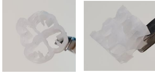
Figure 53. Different views of the carrier material used in SFBBR 1 and 2
