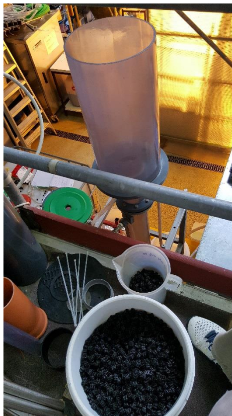
Figure 58. Conditioning of SFBBR-2. Loading of carrier material inside the column
