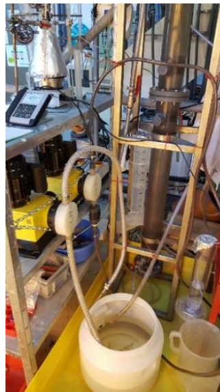
Figure 56. Conditioning of SFBBR-2. Installation of pump system
