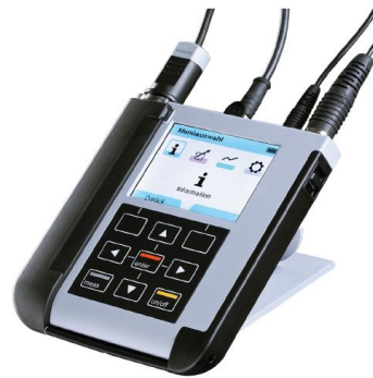
Figure 45. DO sensor – Portavo® 907 MULTI from Knick (Knick, 2017)
