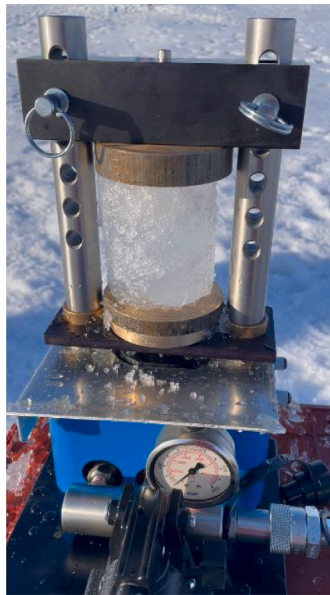
Fig. 2. Compressive load testing device.
