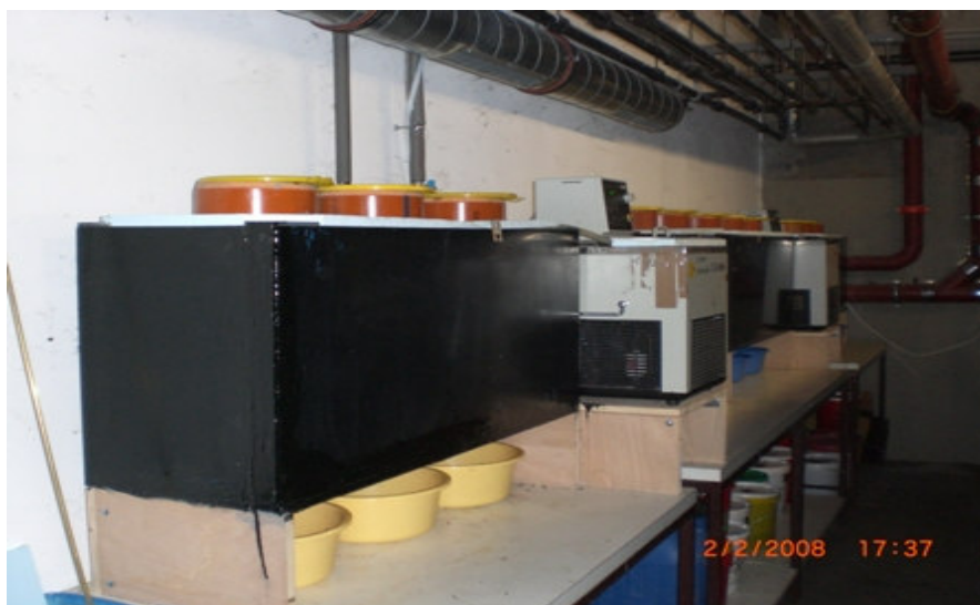
Figure 3.2: Photograph of the continuous flow reactors housed in tanks
