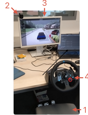
Figure 1: Positioning of the used camera during the study Camera position relative to the test person following numbers define the objects inside the Figure 1: Test Person, 2: Camera, 3: Monitor, 4: Steering wheel
