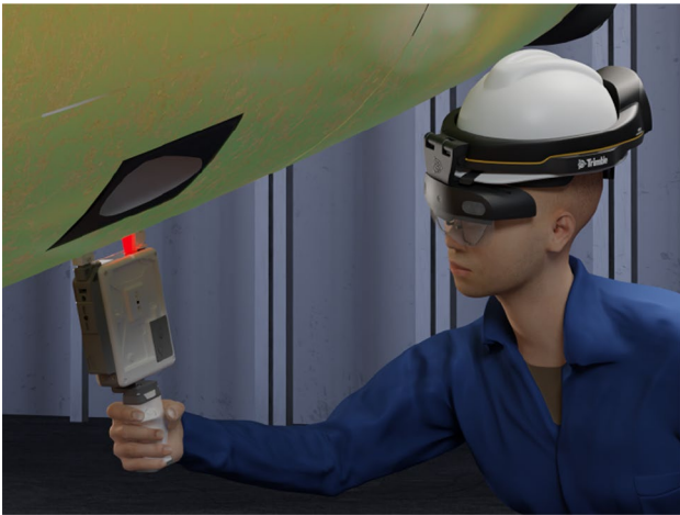
Fig. 7 Manual inspection process of an aircraft fuselage component with digital measuring equipment and assistance by head-mounted Augmented Reality (AR) glasses
