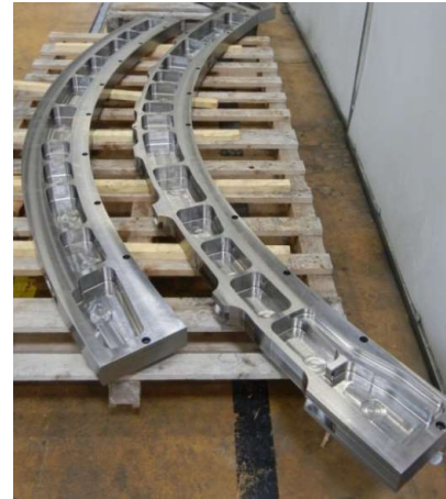
Rough Milling of Pockets
