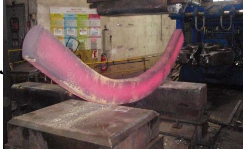
Open Die Forging → Hull Curvature
