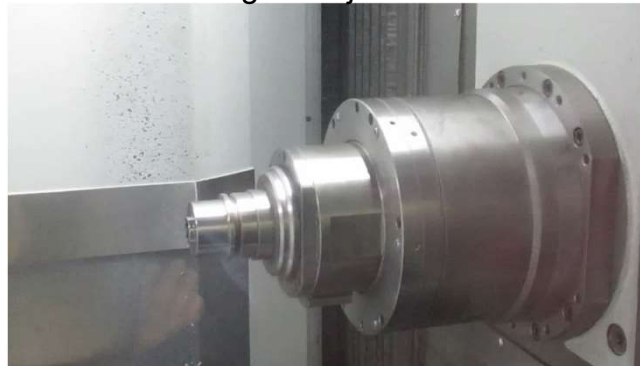
Finish Machining: Jerk j \approx 150\text{ m/s}^3
