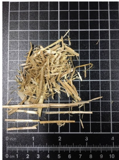
Abb. B.3: Washed wheat straw as used as feed in the experimental investigations.
