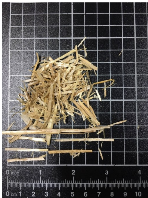
Abb. D.3: Representative sample of the wheat straw used as feed in the experimental investigations (published in 10.1016/j.biortech.2023.130071).
