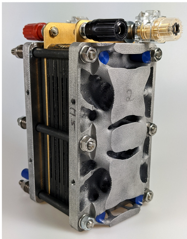
FIG. 7. Photograph of the PEMFC stack assembly with two optimized additively manufactured end plates.
