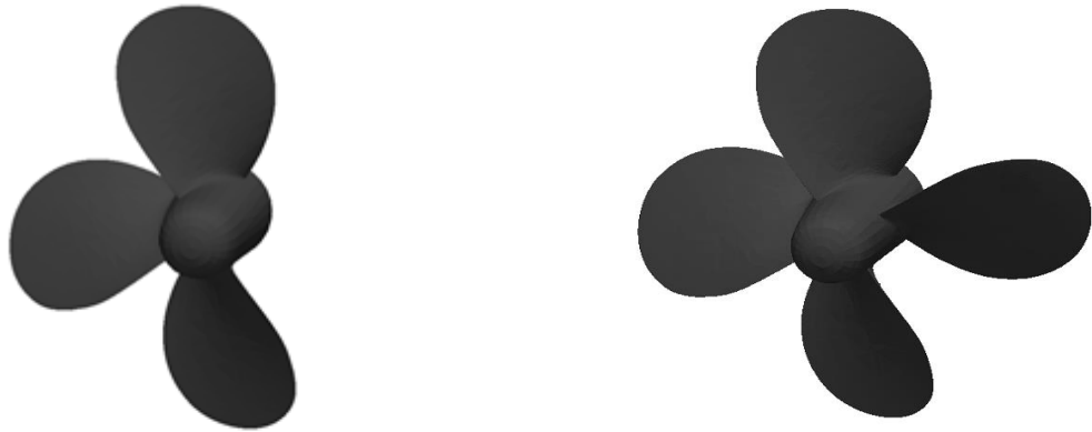
(a) Damaged propeller (b) Four-bladed propeller Figure 1: E779A propeller model
